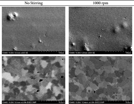
Figure 6.2.2. SEM images showing the structure of SnBi deposits with varying agitation in the bath during deposition (above) and SEM images with electron backscatter that show the detailed grain structure of the deposits (below).
