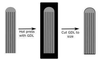
Figure 3.1.4. A diagram of the BPP before hot pressing, after hot pressing with the GDL and after the GDL has been cut to size.
