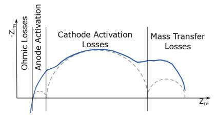
Figure 2.1.9. An example EIS spectrum, showing the features and the corresponding loss mechanism, adapted from [113] and [114].
