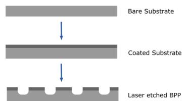
Figure 10.3.2. A diagram of a BPP fabricated by electrodeposition onto the bare substrate, followed by laser etching of the channels, which leaves the coating on the land area.
