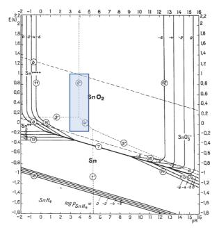
Figure 2.3.1. The Pourbaix diagram for the Sn /  $H_2O$  system at 25 °C, reproduced with permission from [146], and modified to show the operation region of a PEMFC.
