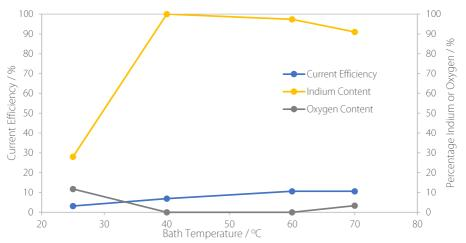
Figure 7.2.19. The influence of the bath temperature on the current efficiency of deposition and the alloy composition of a SnIn alloy.
