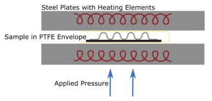
Figure 3.1.3. A diagram of the hot press used to solder the GDL to the BPP through heating under applied pressure.
