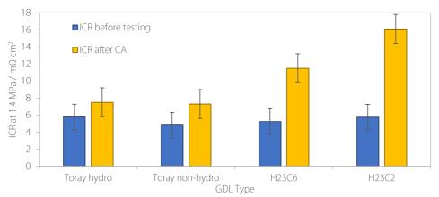
Figure 8.2.6. The ICR for each type of GDL after hot pressing (blue) and after electrochemical testing at 1.0 V<sub>SHE</sub> for 1 hour (yellow).
