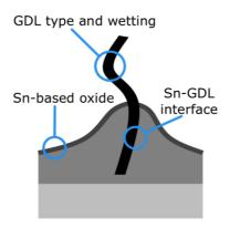
Figure 2.3.5. A diagram showing the areas of interest when designing modifications to the Sn/GDL system
