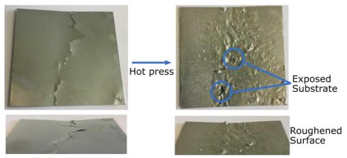
Figure 10.3.1. A series of photographs of a Sn-coated SS316 coupon, having been bent to crack the Sn surface, then hot pressed to repair the damage.
