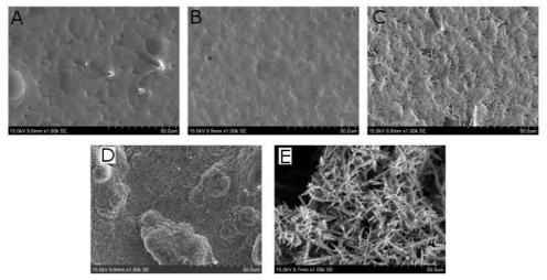
Figure 7.2.6. SEM images of SnIn alloys deposited at various pH. A = -1.0, B = 0.0, C = 1.0, D = 2.0, E = 3.0.
