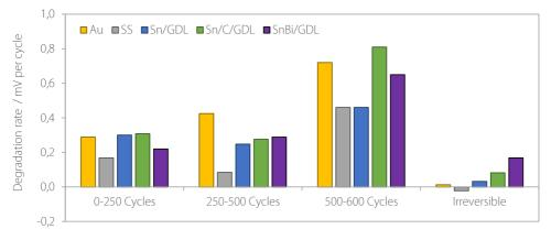
Figure 9.3.6. The degradation rate of each fuel cell during cycling at 1.0 A cm<sup>-2</sup>. Both the reversible degradation rate during each group of drive cycles, and the irreversible rate after the first 500 cycles are shown.
