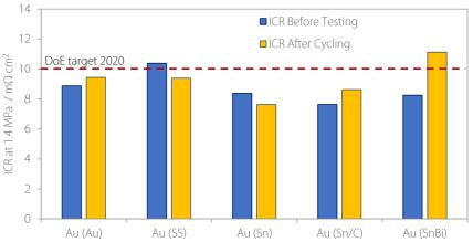
Figure 9.2.1. The *ex-situ* ICR at 1.4 MPa of bipolar plates placed on the anode side of a fuel cell before and after cycling. Each plate was gold-coated stainless steel, and the plate on the cathode side of the fuel cell is indicated in brackets. The red dashed line shows the DoE target for ICR to be reached by 2020.
