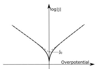
Figure 2.2.2. A visualisation of the Tafel Equation, showing the linear region where the equation is valid, extrapolated to find the exchange current density.
