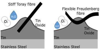
Figure 8.2.4. A drawing of the hypothesised impact of having a stiffer GDL fibre, with the Toray paper going deeper into the Sn layer, forming a larger contact area and therefore a lower ICR.
