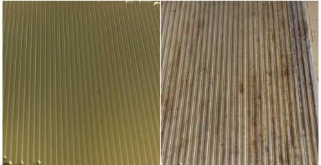
Figure 9.2.2. The flow-fields of a gold coated stainless steel bipolar plate, before (left) and after (right) 200 hours of *in-situ* testing. After testing, there is discolouration on the surface and the coating is faded in places, with brown spots along the channels.
