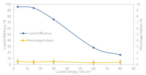
Figure 7.2.2: The influence of the current density of deposition on the current efficiency of deposition and the percentage of indium in the deposit.
