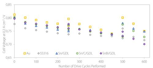
Figure 9.3.2. The progression of the cell voltage at 0.2 A cm<sup>-2</sup> for each fuel cell as the number of drive cycles performed increases.
