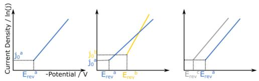
Figure 2.2.3. Kinetics diagrams showing the Tafel slopes for various hypothetical reactions. A comparison of reaction A (blue) with reactions B (yellow) and C (grey) shows that by modifying the applied potential or current, reaction B is favoured over A, however, reaction C is favoured over reaction A at all potentials.
