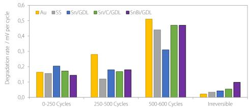
Figure 9.3.3. Average degradation rate of each fuel cell in mV per cycle at 0.2 A cm<sup>-2</sup>. Both the reversible degradation rates in each set of 250 drive cycles, as well as the overall irreversible degradation rate after 500 drive cycles are shown.
