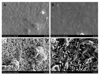
Figure 2.2.10: SEM images showing structure of a Sn layer deposited at various temperatures: A - 20 °C; B - 40 °C; C - 60 °C; D - 80 °C.
