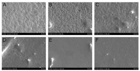
Figure 2.2.11: SEM images of the structure of a Sn layer deposited at various stirring speeds: A - 0 rpm; B - 100 rpm; C - 150 rpm; D - 200 rpm; E - 300 rpm; F - 500 rpm.
