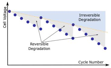
Figure 2.1.8. A typical response of a fuel cell when plotting the cell voltage against cycle number. Regions of reversible degradation are shown in grey, and the irreversible degradation is indicated by the blue region.
