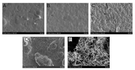
Figure 2.2.9: SEM images of the structure of a Sn layer deposited at various pH: A - pH -1.0; B - pH 0.0; C - pH 1.0; D - pH 2.0; C - pH 3.0.
