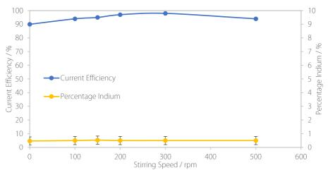
Figure 7.24: The influence of the stirring speed in the bath on the current efficiency of deposition and the amount of indium in the deposit.
