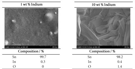
Figure 7.2.8. SEM images and compositions obtained using EDS of two SnIn alloys deposited with 1 wt% (left) and 10 wt% (right) of InCl<sub>3</sub> salt in the bath.
