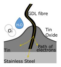
Figure 2.3.2. The Sn/GDL concept, where conductivity is maintained through the GDL fibre, whilst the Tin Oxide provides protection from further corrosion
