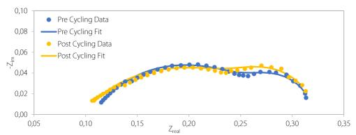
Figure 9.4.5. Nyquist plots showing the measured and fitted impedance of the SnBi/GDL fuel cell before (blue) and after (yellow) 600 drive cycles.
