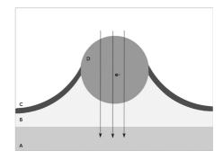
Fig. 1 – The combined Sn/GDL concept. A is the steel bipolar plate, B the deposited Sn, C the SnO<sub>2</sub> layer and D the carbon fibre from the GDL. Electrons can move through the system without obstruction whilst the SnO<sub>2</sub> prevents further oxidation of Sn.
