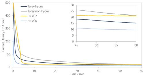
Figure 8.2.5. The current density response of different GDL types during exposure to 1.0  $V_{SHE}$  for 1 hour in a simulated PEM fuel cell environment. The inset shows the final 15 minutes of the test at low current densities.
