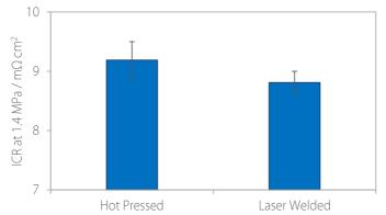
Figure 10.3.4. The ICR of a commercially prepared welded BPP and back plate, compared to a BPP electroplated with Sn and hot pressed to a back plate
