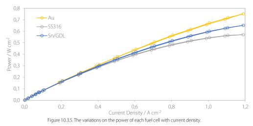
As described in the Strategic Analysis report [294], the commercial BPP has a power density of  $1095 \text{ mW cm}^{-2}$ , which is significantly higher than the performance of the BPPs in this thesis.
