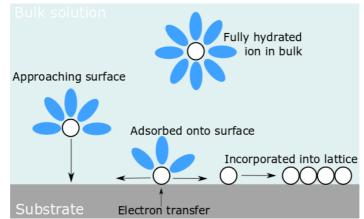
Figure 2.2.5: The stages involved in depositing an atom from the bulk solution to the lattice of a deposit.
