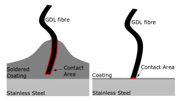
Figure 2.3.4. A diagram showing the difference in contact area between the GDL and coating for two types of BPP. The soldered coating has a significantly higher contact area than the traditional coating method.
