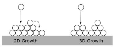
Figure 2.2.7: 2D and 3D growth mechanisms.
