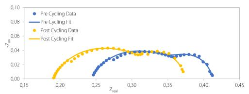
Figure 9.4.3. Nyquist plots showing the measured and fitted impedance of the stainless steel fuel cell before (blue) and after (yellow) 600 drive cycles.
