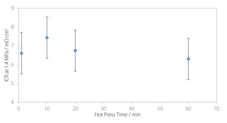
Figure 4.3.4. A comparison of the ICR of bipolar plates hot pressed for varying amounts of time.
