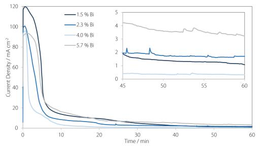
Figure 6.2.4. The current response from SnBi deposits containing various amounts of Bi, during the application of a voltage of  $1.0 V_{SHE}$  over the course of 1 hour in in Na<sub>2</sub>SO<sub>4</sub>/H<sub>2</sub>SO<sub>4</sub> at pH 3 and a temperature of 80 °C. The inset shows a zoom of the final 15 minutes of the current transients.
