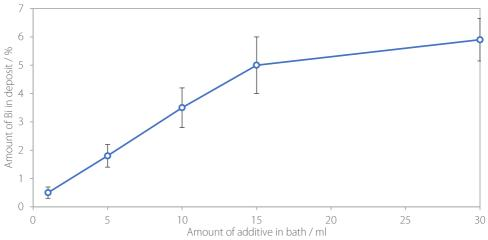
Figure 6.2.1. The relationship between the amount of Slotolet additive in the bath and the bismuth content of the deposit.
