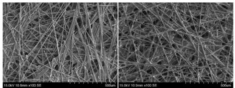
Figure 8.2.3. The two types of Toray paper used in this work, one with a hydrophobic treatment (left) and one without such treatment (right).
