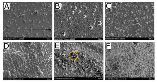
Figure 4.2.1. SEM images of Sn surfaces deposited at varying current densities. a- 7.5 mA cm<sup>-2</sup>; b - 15 mA cm<sup>-2</sup>; c - 30 mA cm<sup>-2</sup>; d - 50 mA cm<sup>-2</sup>; e - 100 mA cm<sup>-2</sup>; f - 150 mA cm<sup>-2</sup>, all images taken before hot pressing. The yellow circle in figure E emphasises the features created by gas eruptions from the substrate.
