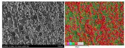
Figure 4.2.2. Zoomed-in SEM images of the sample deposited at 150 mA cm<sup>-2</sup>, with a false colour-EDS image showing the Sn distribution (in red) and the Fe from the bare substrate (in green).
