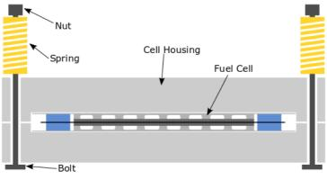
Figure 3.2.3. A cross section of the fuel cell in the cell housing.
