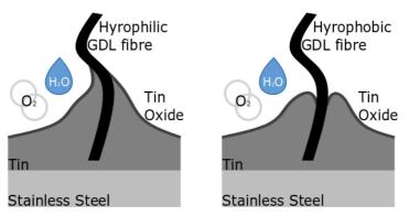
Figure 8.2.2. A drawing of the proposed impact of the PTFE treatment on the wetting properties of the GDL to the Sn, with the hydrophilic GDL having a greater contact area with the Sn than the hydrophobic GDL.
