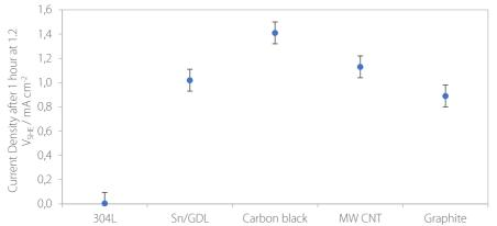
Figure 8.3.6. The corrosion current density of each bipolar plate type after exposure to  $1.2 V_{SHE}$  for 1 hour in a simulated PEMFC environment.
