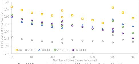
Figure 9.3.5. The progression of the cell voltage at 1.0 A cm<sup>-2</sup> during cycling for each fuel cell.
