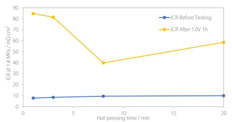
Figure 6.3.3. The ICR of BPPs hot pressed to GDLs for varying amounts of time, before (blue) and after (red) electrochemical tests at 1.0 V<sub>SHE</sub> for 1 hour.
