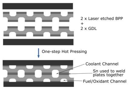
Figure 10.3.3. A summary of the one-step hot pressing procedure used to combine two BPPs and two GDLs to make a single BP/GDL unit that can be combined with a MEA into a fuel cell stack.
