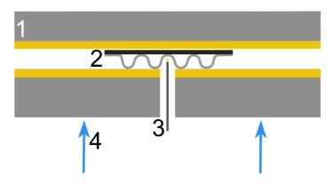
Figure 3.2.1. The setup used to measure Interfacial Contact resistance. 1 is the gold-coated copper plate, 2 is the sample (grey curved line) with GDL (black line), 3 is the gold-coated contact pin, 4 is indicating the presence of a piston used to apply pressure.
