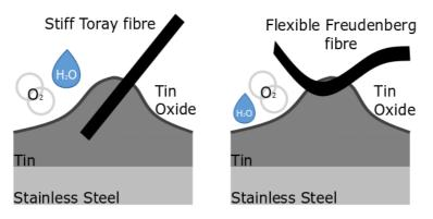
Figure 2.3.6. A diagram showing how the GDL type can affect the interface between the Sn and the GDL, with the stiff Toray fibre penetrating deeper into the Sn than the flexible Freudenberg fibres.
