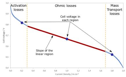
Figure 2.1.7. An annotated polarisation curve showing the dominating loss mechanism in each region. The cell voltage in each region (blue spots) can be mapped over time to determine the fuel cell performance. The resistance of the fuel cell can be estimated by applying Ohm's law to the linear region of the polarisation curve (in red).
