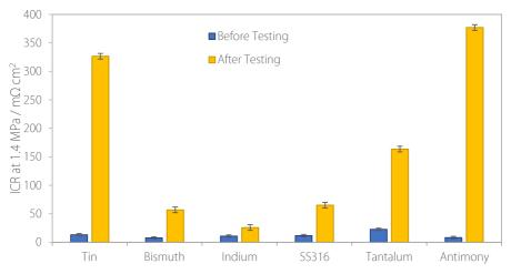
Figure 5.3.1. ICR of the different samples of metal before and after electrochemical testing at 1.0 V<sub>SHE</sub> for 1 hour.
