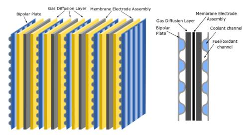
Figure 2.1.2: A schematic diagram of a PEM Fuel Cell Stack, and a single cell
