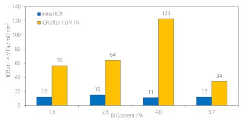
Figure 6.2.5. The ICR of samples with varying bismuth content before (blue) and after (yellow) exposure to  $1.0 V_{SHE}$  for 1 hour in a simulated fuel cell environment.
