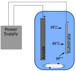
Figure 2.2.1. A standard electrodeposition setup, where an external power supply forces the movement of electrons and metal ions from the electrolyte to the cathode (substrate), where they are reduced to form a layer of metal.
