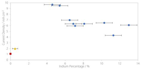
Figure 7.3.3. The influence of the Indium content on the final current density of a sample after being held at 1.0  $V_{SHE}$  for 1 hour. The blue circles are hot-dipped SnIn samples of varying In content, the yellow triangle is an electroplated SnIn sample, and the red square is an electroplated Sn sample.
