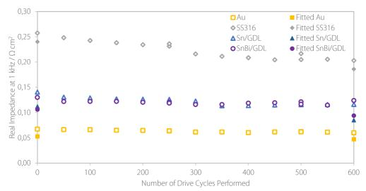
Figure 9.4.1. The real impedance of each fuel cell at 1 kHz, plotted over cycle number (unfilled shaped). The fitted HFR at 0 and 600 cycles (filled shapes) is also plotted for comparison.
