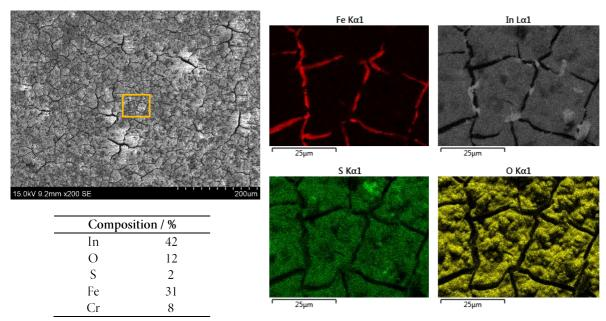
Figure 7.2.14. A SEM image of a sample of SnIn deposited onto a glass-blasted substrate at 60 °C, with EDS analysis showing the Iron (Fe, red), Indium (In, grey), Sulfur (S, green) and Oxygen (O, yellow) distribution. The yellow box on the SEM image indicates the area analysed by EDS, and the table shows the percentage composition of the area analysed by EDS.
