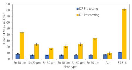
Figure 4.2.5. A comparison of the ICR of bipolar plates with varying thickness Sn layer hot pressed to a GDL, before and after *exsitu* electrochemical testing for 1 hour at 1.0 V<sub>SHE</sub>.
