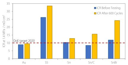
Figure 9.2.3. The ICR of bipolar plates placed on the cathode side of the fuel cell, before and after 600 drive cycles. The red dashed line shows the DoE target for ICR to be reached by 2020.
