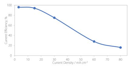
Figure 2.2.12: The effect of current density on the current efficiency of deposition, for the deposition of Sn from a sulphate bath at 25 °C.
