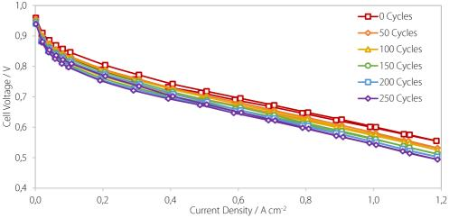
Figure 9.3.1. An example of the progression of polarisation curves with increasing numbers of drive cycles.
