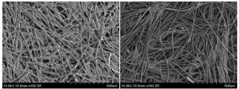
Figure 8.2.1. The two types of Freudenberg H23 papers used in this thesis. The H23 C6 paper that has been given a hydrophobic treatment to the carbon fibres (left) and the H23 C2 paper that has not received any treatment (right).
