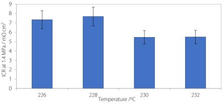
Figure 4.3.2. The correlation between the hot pressing temperature of a BPP and its ICR.
