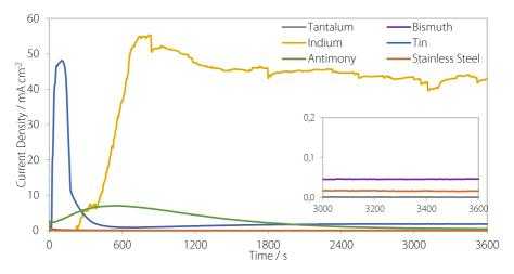
Figure 5.2.1. The current density response for pure metals exposed to 1.0 V<sub>SHE</sub> for one hour, with the inset showing a zoomed in section at very low current densities for the last 10 minutes.
