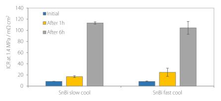
Figure 6.3.5. The ICR for slowly and quickly cooled bipolar plates after pressing (blue), after 1 hour of electrochemical testing (yellow) and after 6 hours of electrochemical testing (grey).
