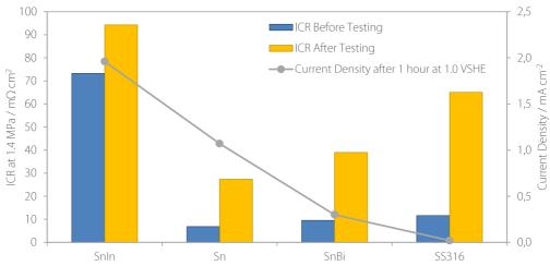
Figure 7.2.21. The interfacial contact resistance of the SnIn coating before (blue) and after (yellow) electrochemical testing as compared to the bare stainless steel (SS316), Sn coated and SnBi coated steel plates, with the final current density (grey) after 1 hour of chronoamperometric testing at 1.0 V<sub>SHE</sub>.
