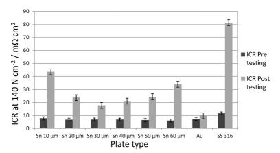
Fig. 4 - Comparison of coating thickness against ICR before and after ex-situ testing.
