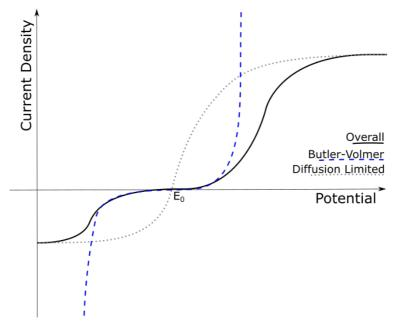
Figure 2.24. A characteristic current density profile showing the overpotential regions limited by mass transport (diffusion) and electron transport (Butler Volmer).
