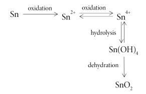
Figure 4.4.1. An overview of the corrosion and passivation processes occurring on a Sn surface in an acidic environment [191].
