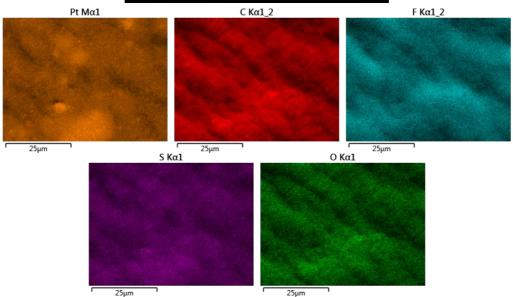
Figure 9.5.1. A SEM image of the MEA from the Stainless Steel fuel cell (top), with EDS analysis of the area to show the distribution of platinum (orange), carbon (red) fluorine (teal), sulfur (purple) and oxygen (green).
