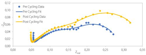
Figure 9.4.2. Nyquist plots showing the measured and fitted impedance of the gold coated BPP fuel cell before (blue) and after (yellow) 600 drive cycles.
