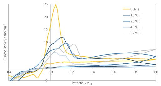
Figure 6.2.3. Cyclic voltammograms of samples of Sn containing between 0 and 6 % Bi when swept between -0.4 and 1.0  $V_{SHE}$  at 1 mV s<sup>-1</sup> in Na<sub>2</sub>SO<sub>4</sub>/H<sub>2</sub>SO<sub>4</sub> at pH 3 and a temperature of 80 °C. Three cycles were performed, and the final cycle for each sample is shown here.
