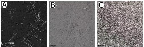
Figure 8.3.4. Light Microscope images of a GDL sprayed with around 0.2 mg cm<sup>-1</sup> of A: Carbon Black, B: Multiwalled Carbon Nanotubes, C: Graphite.
