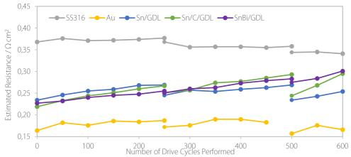
Figure 9.3.7. The estimated resistance from the slope of the ohmic region of the polarisation curve for each cell plotted against the number of drive cycles performed.
