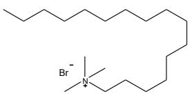
Figure 7.2.15: The structure of cetyl trimethylammonium bromide.
