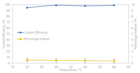
Figure 7.2.3: The influence of the temperature of the deposition bath on the current efficiency of deposition and the amount of indium in the deposit.
