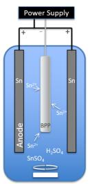
Figure 3.1.2. A diagram of the electrodeposition setup, showing the two Sn anodes, suspended on either side of the stainless steel substrate, in a sulfuric acid based electrolyte.
