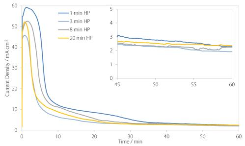
Figure 6.3.2. The current response of SnBi samples that have been hot pressed for various amounts of time without a GDL present, when exposed to  $1.0 V_{SHE}$  for 1 hour in a simulated PEMFC environment.
