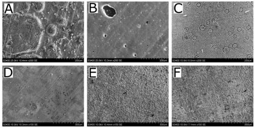
Figure 4.2.3. SEM images of Sn surfaces deposited at varying current densities. a - 7.5 mA cm<sup>-2</sup>; b - 15 mA cm<sup>-2</sup>; c - 30 mA cm<sup>-2</sup>; d - 50 mA cm<sup>-2</sup>; e - 100 mA cm<sup>-2</sup>; f - 150 mA cm<sup>-2</sup>, all images taken after hot pressing.
