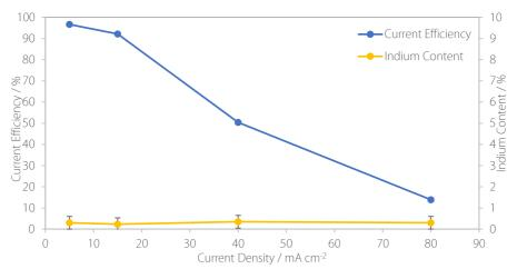
Figure 7.2.9. The influence of current density of deposition on the amount of indium in a Sn deposit and the current efficiency of deposition.
