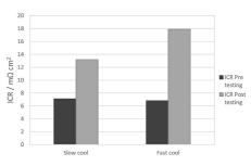
Fig. 3 – Comparison of the quickly vs slowly cooled plates before and after corrosion testing.
