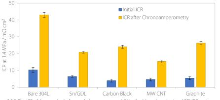
Figure 8.3.5. The ICR of the samples before and after exposure to 1.2  $V_{SHE}$  for 1 hour in a simulated PEMFC environment.
