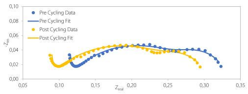
Figure 9.4.4. Nyquist plots showing the measured and fitted impedance of the Sn/GDL fuel cell before (blue) and after (yellow) 600 drive cycles.
