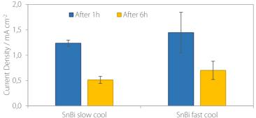
Figure 6.3.4. The current density of slowly and quickly cooled SnBi BPPs after one hour (blue) or six hours (yellow) of an applied potential of 1.0 V SHE in a simulated PEMFC environment.
