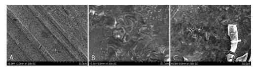
Figure 7.2.18. SEM images of SnIn samples deposited at A - 5, B - 10, and C - 20 mA cm<sup>-2</sup>.
