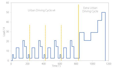
Figure 2.1.6. A single drive cycle used for *in-situ* fuel cell testing, consisting of four short urban driving cycles followed by an extra-urban driving cycle
