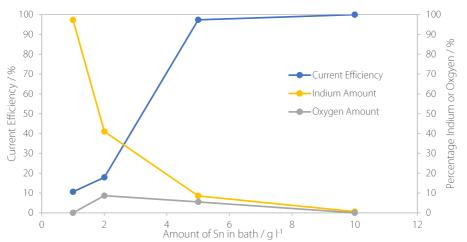
Figure 7.2.20. The influence of the Sn content of the bath on the current efficiency of deposition at 15 mA cm<sup>-2</sup> and 60 °C, and the deposit composition of a SnIn alloy.
