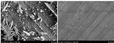
Figure 2.2.8: SEM images of the structure of a Sn layer deposited A - without and B – with levelling and brightening agents.
