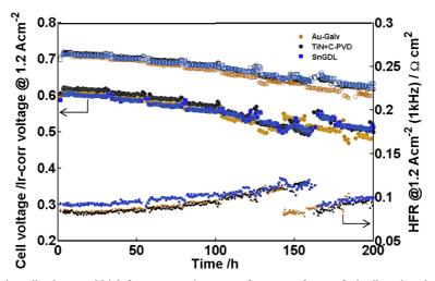
Fig. 7 - 200 h in-situ cell voltage and high frequency resistance performance of a PEM fuel cell equipped with Au (yellow circles), TiN + C (black circles) and Sn/GDL (blue squares) BPPs. (For interpretation of the references to color in this figure legend, the reader is referred to the Web version of this article.)
