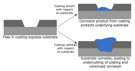
Figure 10.2.1. The two possible corrosion processes when the substrate is exposed. If the coating is anodic with respect to the substrate, the coating will start to corrode, producing a corrosion product that passivates the surface. If the coating is cathodic with respect to the substrate, the coating will not corrode, but the substrate will begin to corrode underneath the coating, producing a large amount of corrosion products and deep pits.
