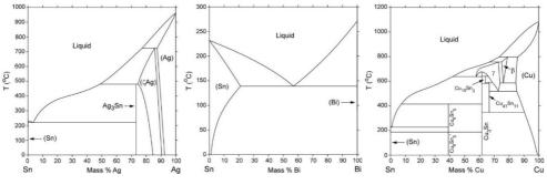
Figure 2.2.13: Phase diagrams of binary Sn alloys. A, SnAg [139]; B, SnBi [140]; C, SnCu [141].
