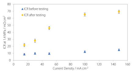
Figure 4.2.4. Comparison of current density of deposition against the ICR measured before and after *ex-situ* electrochemical testing.
