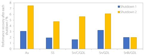
Figure 9.3.4. The recovery of each fuel cell after the first and second shutdowns as a percentage of the initial cell performance.
