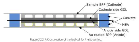
The fuel cell was placed inside a custom-made cell housing from ElringKlinger, and a pressure of 1.4 MPa was applied as shown in Figure 3.2.3, using four springs, one in each corner. The cell was then connected up to a Greenlight G40 test station in counter flow configuration.
