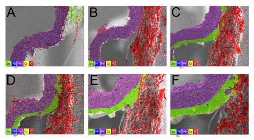
Figure 4.2.6. Cross-sectional EDS images of BPPs & GDL with varying thickness of Sn after *ex-situ* testing, purple representing the Fe in the bipolar plate, green the Sn and red the C in the GDL. The initial thickness of deposits was 10, 20, 30, 40, 50 and 60  $\mu$ m on figure a to f respectively.
