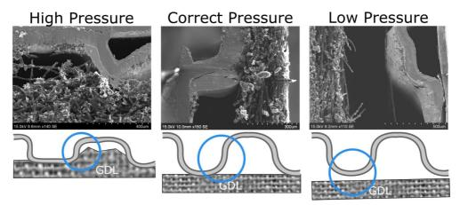
Figure 4.3.1. SEM images and figures of BPPs hot pressed at varying pressures.
