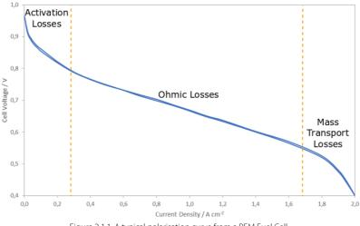
Figure 2.1.1. A typical polarisation curve from a PEM Fuel Cell.
