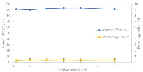
Figure 7.2.1: The influence of the amount of additive present in the bath on the current efficiency of deposition and indium percentage in the deposit. The error bars in indium percentage reflects the uncertainty in the EDS measurements.
