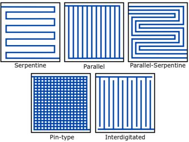
Figure 2.1.3. A diagram showing the most common types of flow fields for bipolar plates
