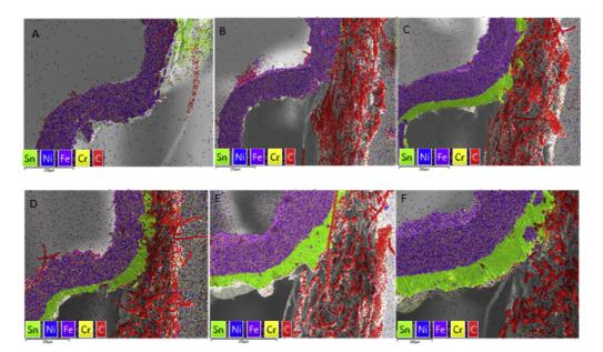
Fig. 5 – Cross-sectional EDS images of BPPs & GDL with varying thickness of Sn after ex-situ testing, purple representing the bipolar plate, green the Sn and red the GDL. The initial thickness of deposits was 10, 20, 30, 40, 50 and 60  $\mu$ m on figure A to F respectively. (For interpretation of the references to color in this figure legend, the reader is referred to the Web version of this article.)
