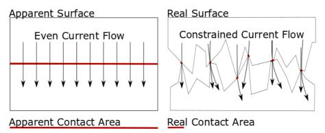
Figure 2.3.3. A diagram showing how the real surface differs from the apparent surface, leading to a much smaller 'real' contact area and a constrained current flow.
