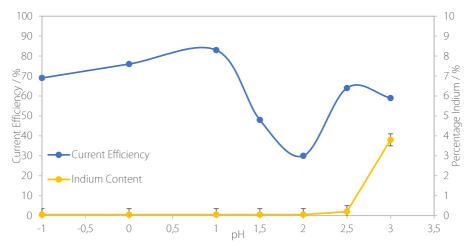
Figure 7.2.5: The influence of the pH of the deposition bath on the current efficiency of deposition and the amount of indium in the deposit.
