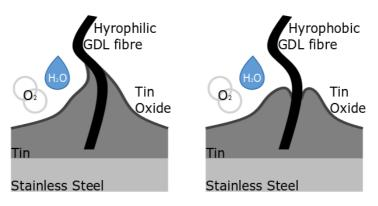
Figure 2.3.7. A diagram showing how the hydrophobicity of the GDL fibre will affect its contact with the Sn, with the hydrophilic GDL fibre, left, predicted to have better contact with the Sn than the hydrophobic GDL fibre, right.
