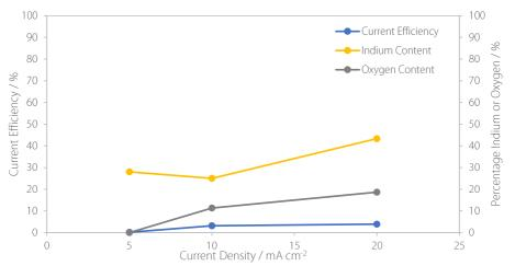
Figure 7.2.17: The influence of the current density of deposition on the current efficiency of deposition and the composition of the electrodeposited SnIn alloy.
