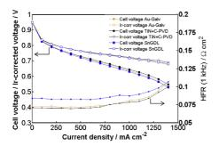
Fig. 6 – Beginning of life performance of the fuel cell equipped with Au (yellow) TiN + C (black) and Sn/GDL (blue) bipolar plates. (For interpretation of the references to color in this figure legend, the reader is referred to the Web version of this article.)
