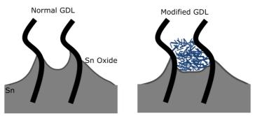
Figure 8.3.2. A drawing of the Sn/GDL interface unmodified (left) and modified with carbon (right) to block the movement of Sn into the GDL and reduce the surface area exposed to electrolyte.
