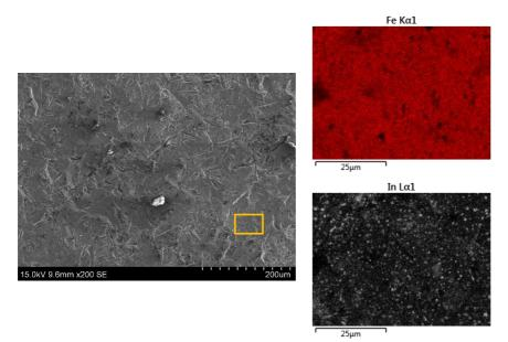
Figure 7.2.13. A SEM image of a sample of SnIn deposited onto a glass-blasted substrate at 40  $^{\circ}$ C, with EDS analysis showing the Iron (Fe) distribution in red and the Indium (In) distribution in white. The yellow box on the SEM image indicates the area analysed by EDS.
