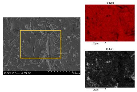
Figure 7.2.12. A SEM image of a sample of SnIn deposited onto a glass-blasted substrate at 20°C, with EDS analysis showing the Iron (Fe) and Indium (In) distribution. The yellow box on the SEM image indicates the area analysed by EDS.
