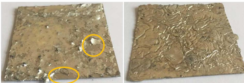
Figure 7.3.1. Photographs of a SnIn layer hot-dipped onto a stainless steel coupon before (left) and after (right) heating to 226 °C. Before heating, bare substrate is visible (yellow circles) and the surface is very rough, but after heating the substrate is completely covered and the surface is smoother.
