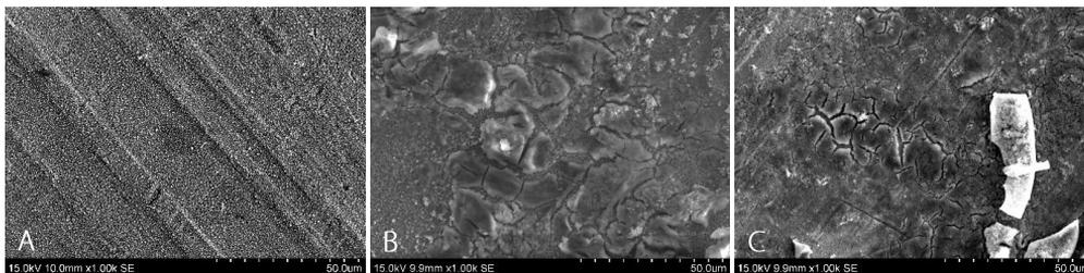
Figure 7.2.18. SEM images of SnIn samples deposited at A - 5, B - 10, and C - 20 mA cm<sup>-2</sup>.
