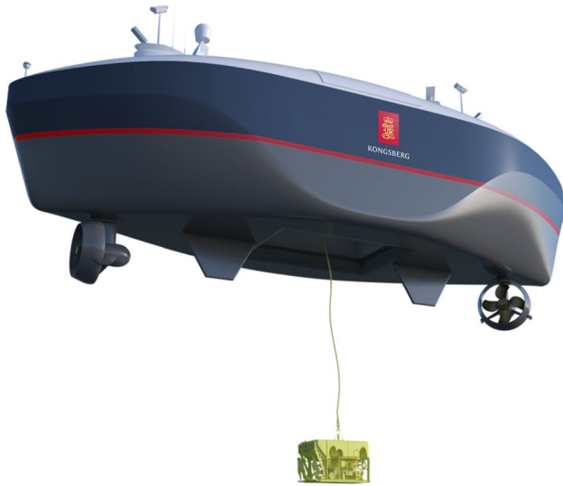
Fig. 1 Exemplar illustration of the ROV launched and recovered from a relatively small USV. Courtesy Kongsberg Maritime
