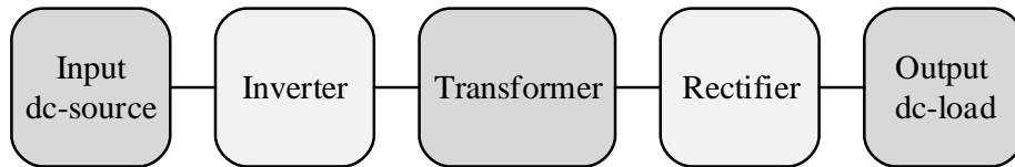
Figure 3.1: Block diagram of the converter structure, where the topic of the chapter, the inverter and rectifier, are highlighted.
