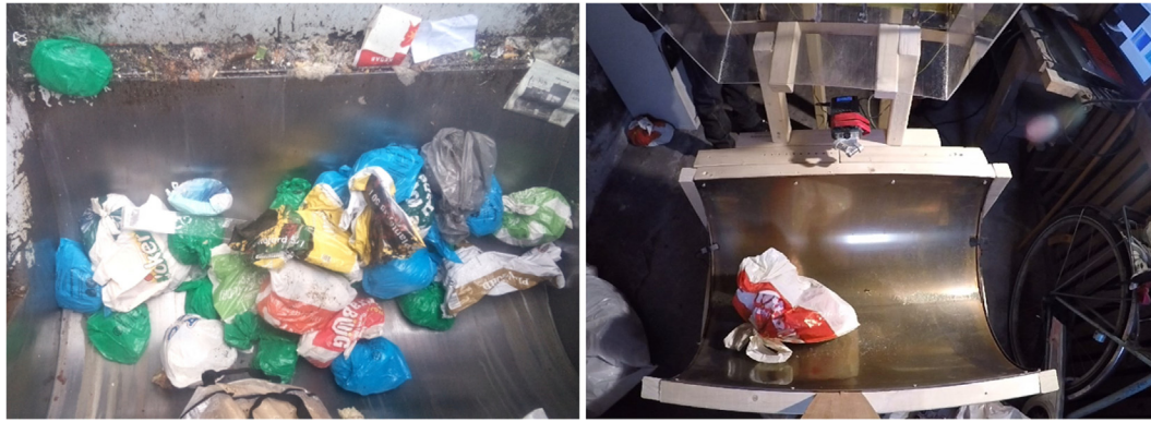
Fig. 1. The landing tray of a waste collection truck during operation on the left and the test rig on the right.
