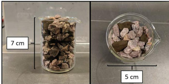
Figure 3.14: Sample in beaker with diameter similar to crucible diameter. Picture shows Comilog ore mixed with quartz in 1:1 ratio according to weight
