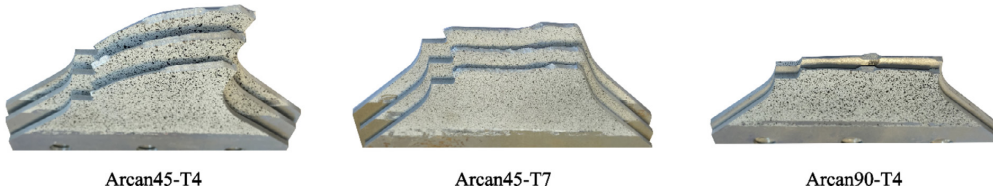
Fig. 10. Fractured specimens showing the different fracture modes of the modified Arcan tests with corresponding fracture surfaces.
