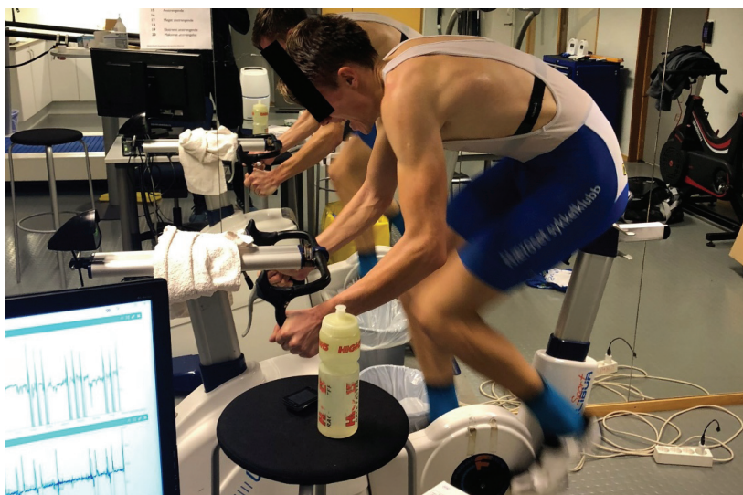
Figure 7: Example of sprint in the seated position on a Lode Excalibur Sport electromagnetic braked cycle ergometer.
