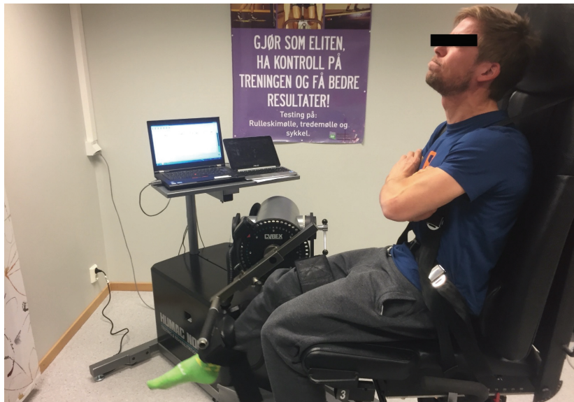
Figure 10: Example of one-legged isokinetic knee extension test performed 24 hrs after the 4-h experimental protocol using the Humac Norm dynamometer.
