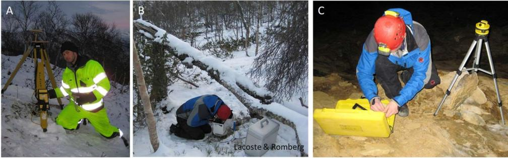
Figure 5 Glimpses of fieldwork during field season 2007. A: Kjetil Broberg next to the dGPS total station at the Svarthammar plateau. B: Terje Solbakk reading the Lacoste&Romberg gravimeter. C: Terje Solbakk mounting gear for cave profile surveying. Photos: A: Terje Solbakk, B and C: Kjetil Broberg.
