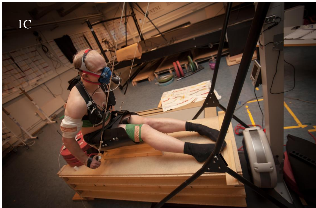
Figure 1: 1A: Picture of the modified poling ergometer with the ice sledge-hockey seat mounted to a platform. The red rings are marking the positions of the reflective markers used with the Qualisys Oqus camera-system. 1B: Picture of the force cell mounted inside the ergometer. 1C: Picture of an athlete using the ergometer.
