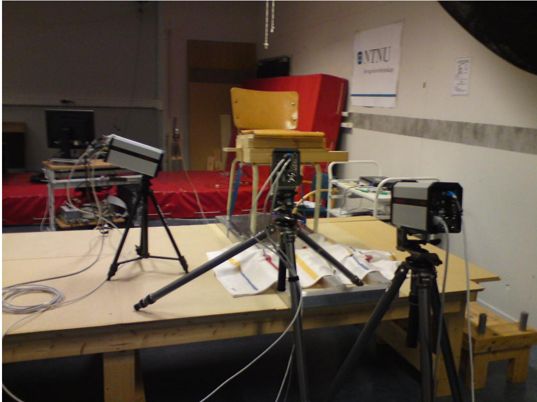
Picture 2: Frontal view of chair and motion capture cameras, with pulley visible in the background
