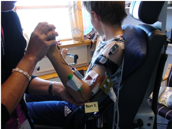
Figure 1. Experimental setup with EMG sensors, goniometer and accelerometer placed on the arm
