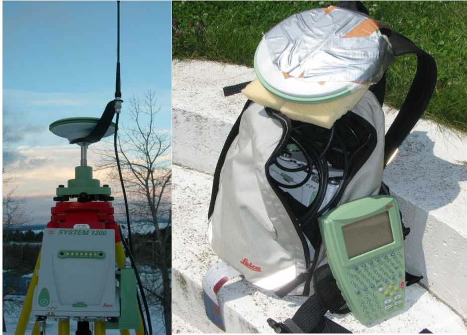
Figure 3. The d-GNSS used in study V . The reference station is shown on the left side, and the backpack carried by the athlete is shown on the right side.
