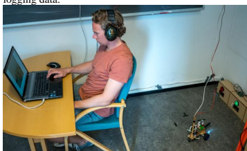
Figure 3. Experiment setup. The participant can only see the robot through the display provided on the laptop screen, which is a first-person camera view.
