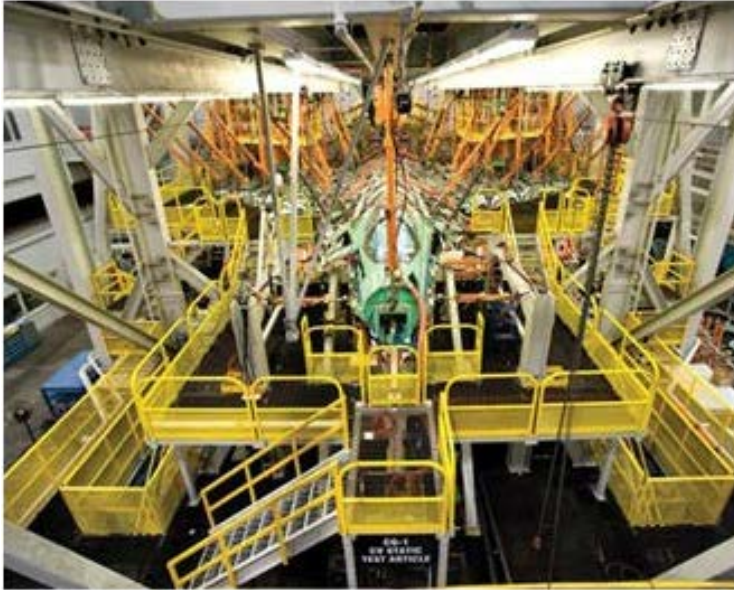
Figure 3: F-35 in a testing frame.
