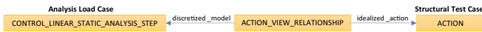
Fig. 14. Load cases from the Analysis data set are related to the Test Case of the Structural Test data set via the action_view_relationship.
