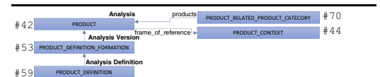
Fig. 6. Left: Extract of a STEP P21 file. Right: Graphical representation used in this paper.
