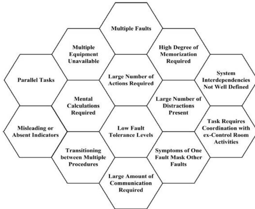
Figure 3. Factors contributing to complexity in SPAR-H (Gertman et al., 2005).
