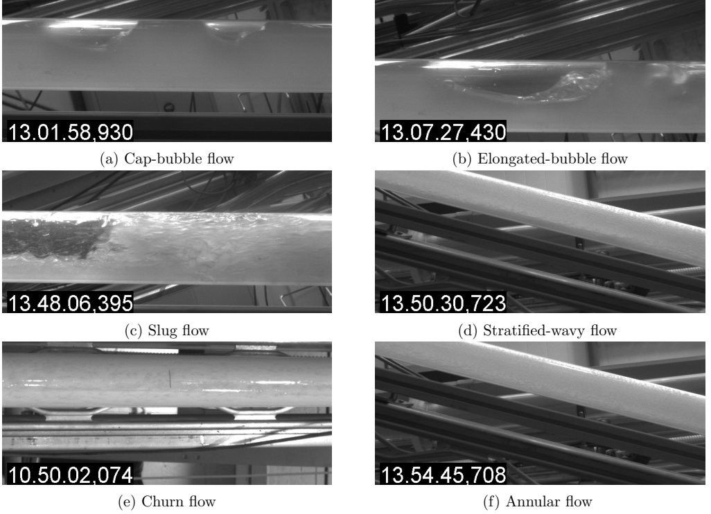
Figure 3.13. Classification criteria for flow patterns
