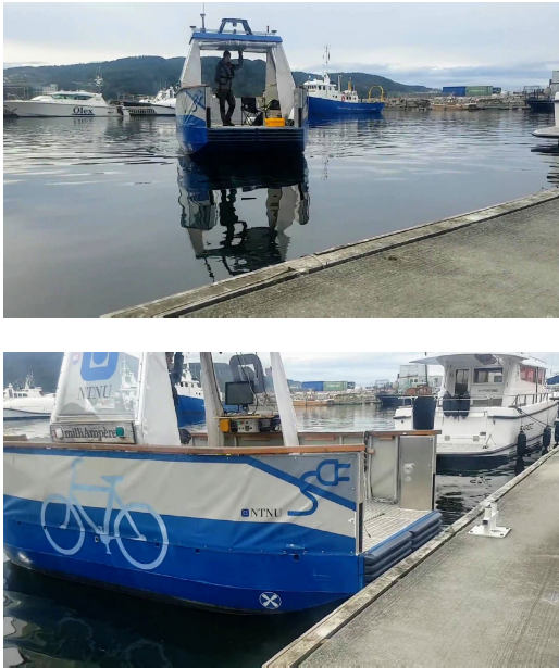
FIGURE 15. The milliAmpere while performing the docking maneuver, including closing in on the dock, and the final docking pose.
