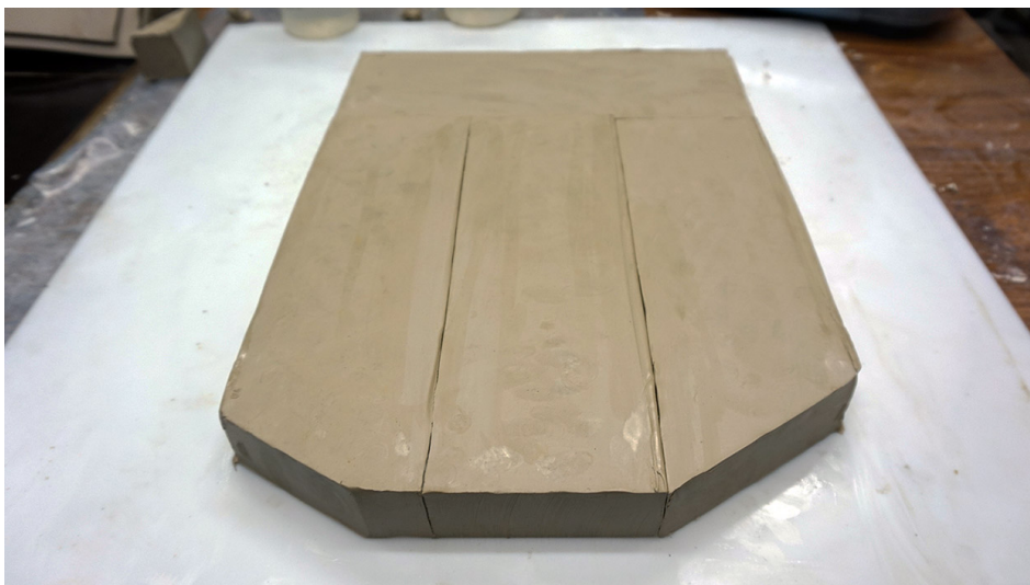
Figure A.35. A 4cm thick Type 2 clay layer.
