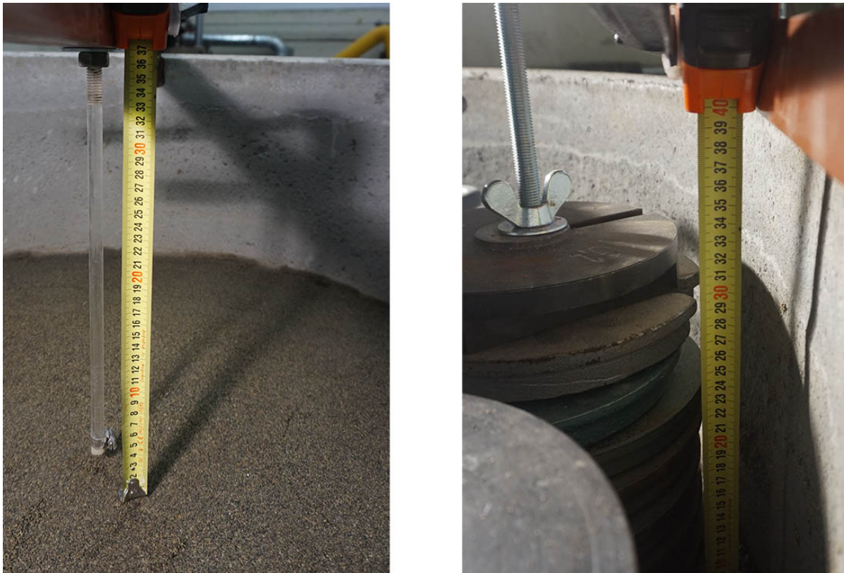
Figure A.46. Compaction of top of sample due to the dead weight plate. Left: Before. Right: After.
