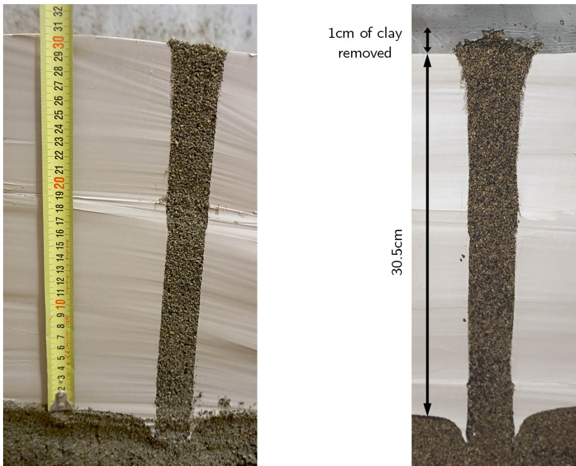
Figure A.51. Section cut of the 31.5cm clay layer of Case A. 1cm of clay was removed on the top of the sample.
