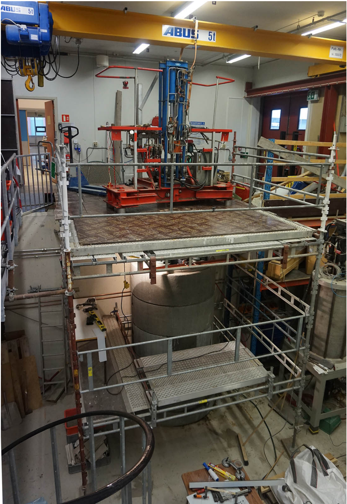
Figure A.56. Image of the chamber, platform and bore rig
