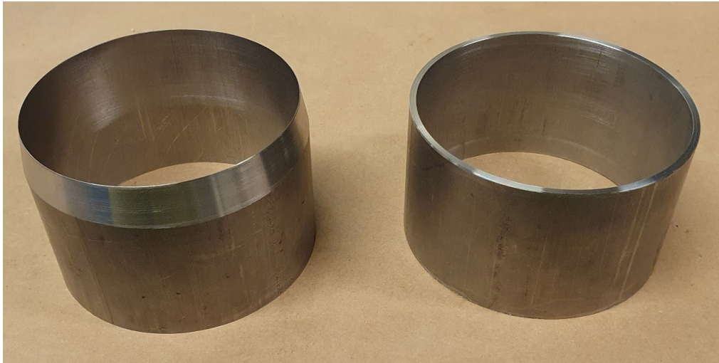
Figure A.40. Density sampler ring, 7.2cm diameter and 5cm height, with an extension to the right.
