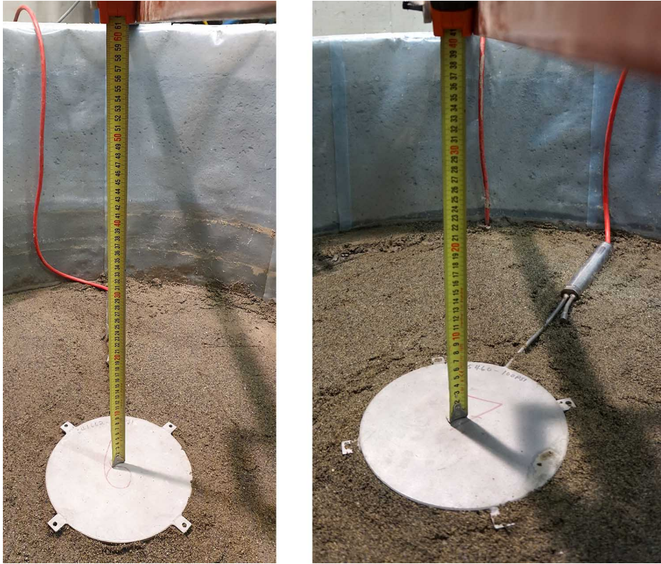
Figure A.57. The local depths of the two earth pressure sensors in the sample
