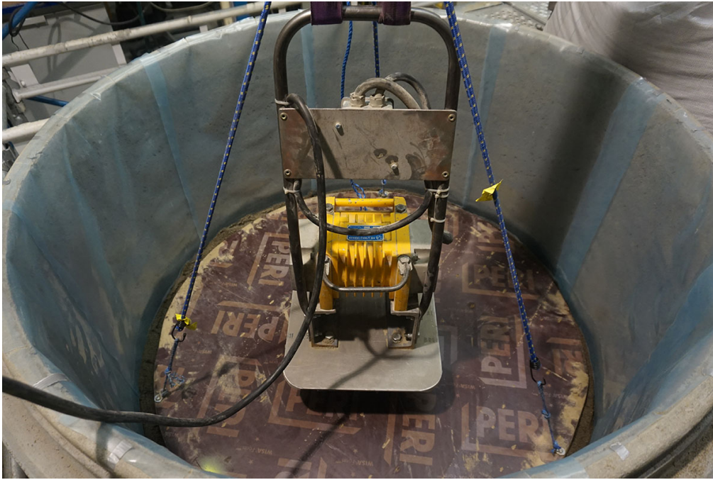
Figure A.31. Equipment used for compaction of sand.
