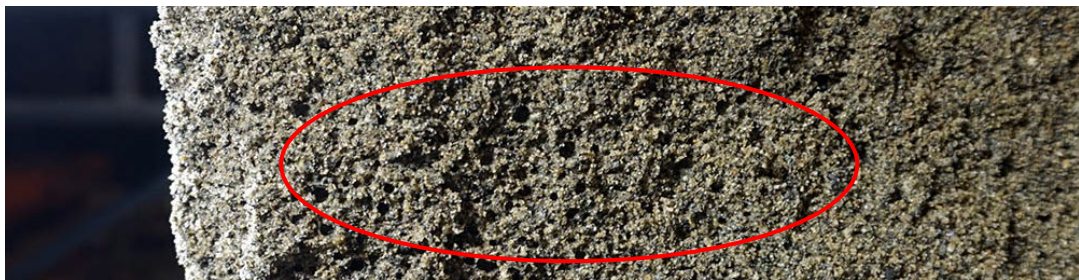
Figure A.68. Local spherical voids in the sand.
