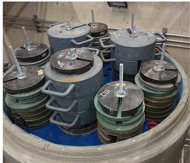
Figure A.55. Left: Levelled surface on top of sample. Right: Added dead weight plate
