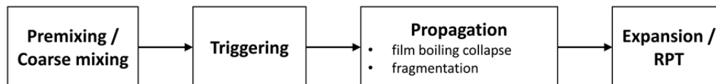
Figure 2: four steps for the water-molten metal RPT adapted from (Shen et al., 2018).
