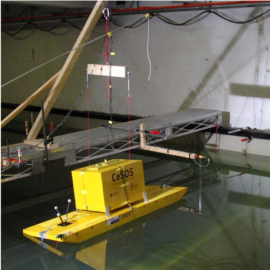
Figure D.5: Barge model with the arrangement for the free decay test in rolling
