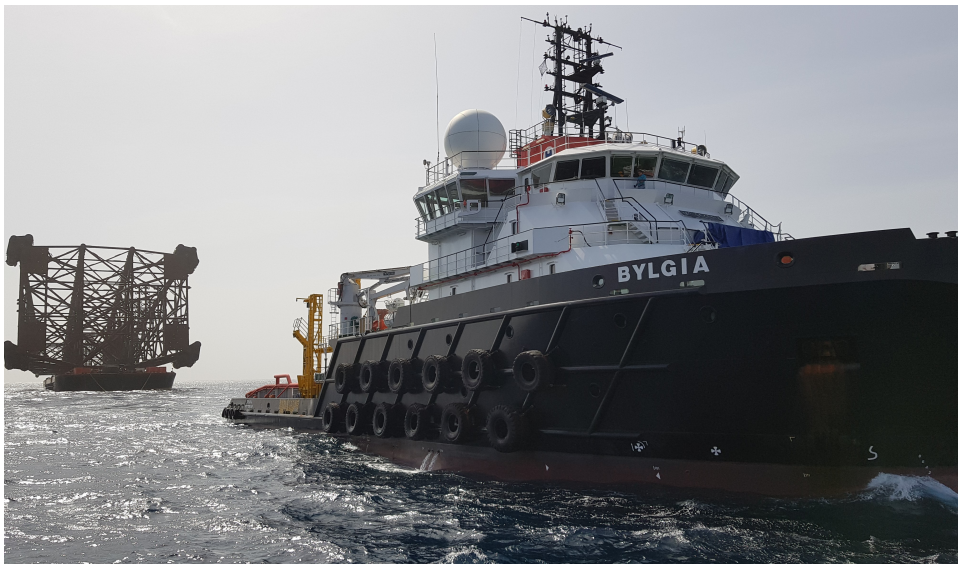
Figure 1.2: A typical heavy transport; transport of the Peregrino jacket on the barge H-542 towed by the tug Bylgia from the Netherlands to Brazil in November 2019 (the picture is taken during an inspection of the barge and cargo; during offshore tow, the tow line is much longer). Photo: Asle Natskår.
