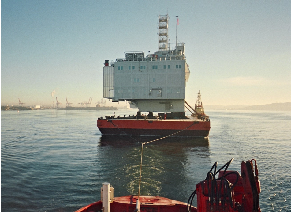
Figure 3.2: A Standard North Sea barge loaded with the Living Quarter to the Kristin platform, towed from Gothenburg, Sweden, to Stord, Norway in 2005. The barge is seen from the tug Bamse. The picture is taken during tow out of the harbor; during offshore tow, the tow line is much longer. Photo: Asle Natskår.
