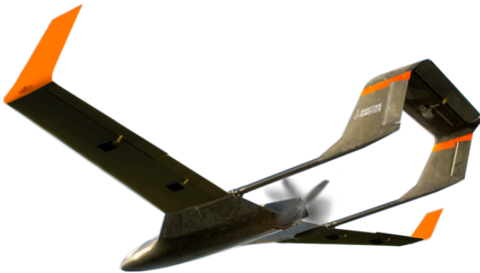
Fig. 7. P31016 concept battery-powered fixed-wing unmanned aircraft
