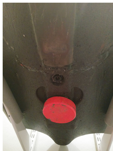
Fig. 9 The object to be released attached to the underside of the UAV's fuselage
