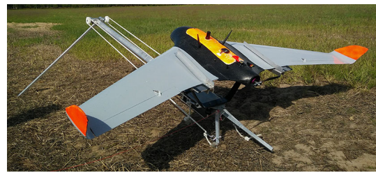
Fig. 6 The UAV used in the case study, placed in its launcher
