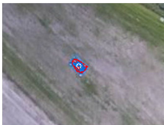
Fig. 4 The resulting processed image with the detection marked. The red areas mark the detected contours and the white circle marks the center of detection that is used for georeferencing. Notice that multiple red contours are displayed in the image, and that contours within contours are removed after this image is generated so that only the largest contour remains (Color figure online)
