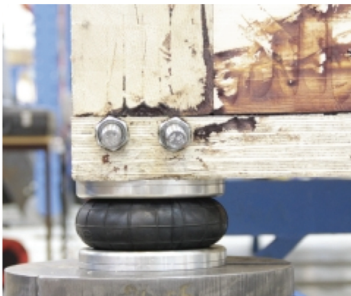
Fig. 4. Free-free boundary conditions: detail showing the air bellows.
