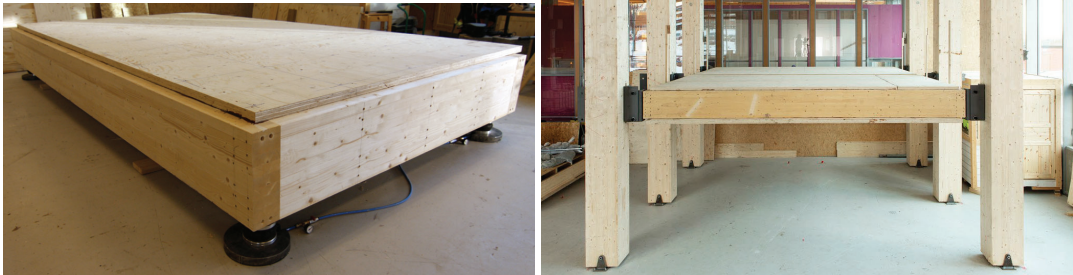
Figure 3: The two experimental setups: LEFT (a): Element L1 mounted on air bellows; setup used for the free-free BC measurements. RIGHT (b): Woodsol prototype ; setup used for the on columns BC measurements (foto:SINTEF/Anne-Line Bakken).
