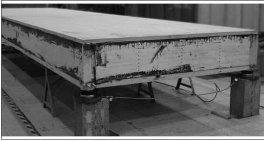
Figure 2. Woodsol floor element installed on air bellows.
