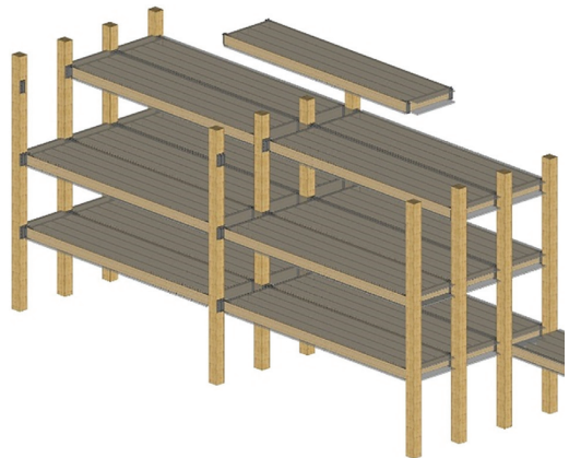
Fig. 1. Woodsol building system: frame construction based on moment resisting connection between continuous columns and stiff floor elements [11].
