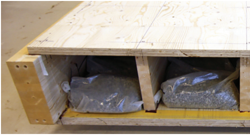
Fig. 6. Element cavity with the gravel bags.
