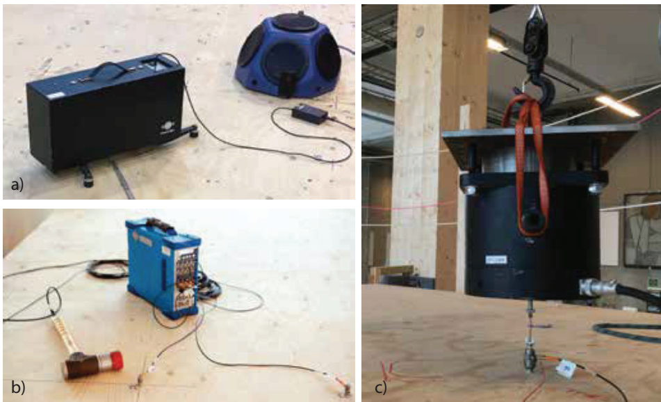
Figure 2.6. Excitation sources. a) Tapping machine and semi-dodecahedron. b) Impact hammer with acquisition system. c) Shaker with impedance head.
