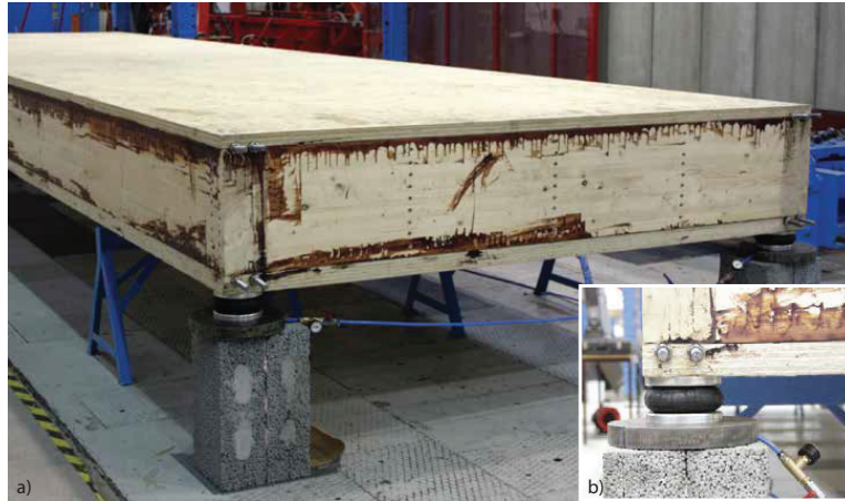
Figure 2.3. Experimental setup with free-free boundary conditions. a) 9 m floor element on air bellows. b) Detail of the air bellows.
