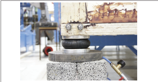
Figure 3. Detail of the supporting air bellows.
