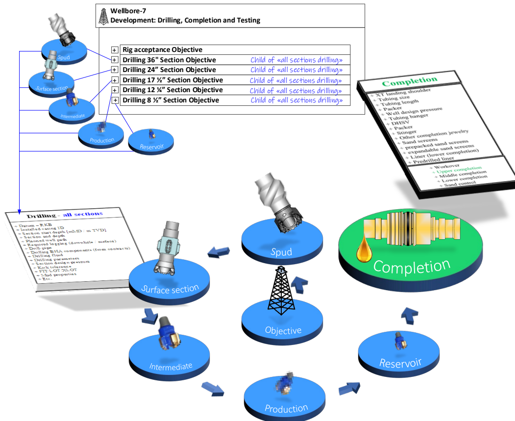
Figure 3-8- Each section drilled use the "parent" for every well, while completion apply the parent once.
