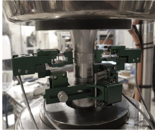
Figure 7: Illustration of the axial-torsional extensometer mounted on a test specimen
