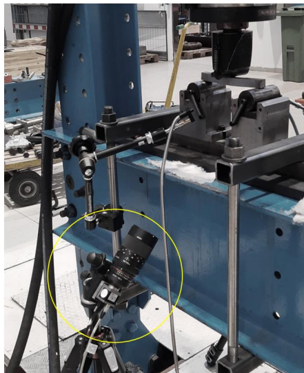
Figure 10: The DIC camera setup, one camera on either side of the specimen
