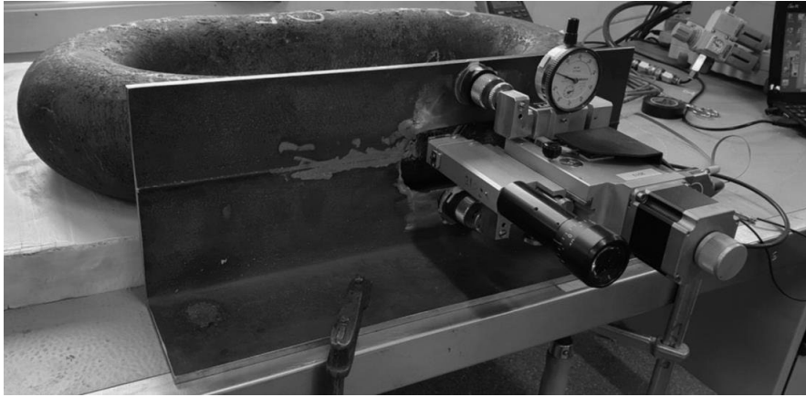
Figure 12: The HD experimental setup. Due to the limited space between the chain straight parts, only RS at the chain outer surface were measurements using the HD technique
