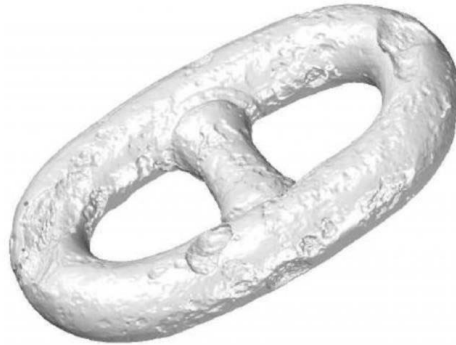
Figure 3: 3D scan of a studlink retrieved from service, courtesy of [17]
