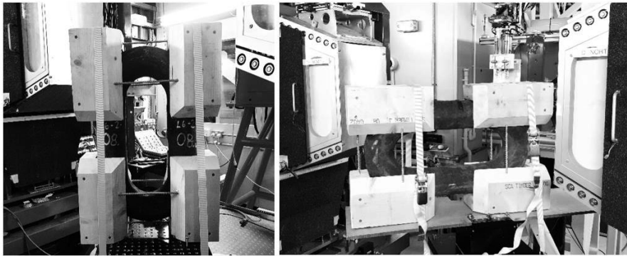
Figure 13: The ND experimental setup. The links are repositioned to enable the 3-axis RS measurement, courtesy of [74]
