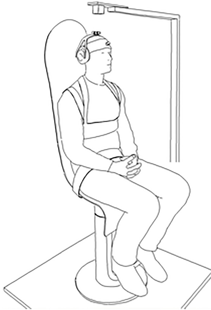
Fig 1. An instrumented participant strapped to the actuated chair. Sensors were placed on the chair, on the back of the subject at the level of the 2 nd thoracic vertebrae, and on the forehead. The electromagnetic transmitter was placed ~20 cm above the head of the subject. Earmuffs have holes leaving the ears uncovered and hearing intact. Supporting information for the set up can be found in Stensdotter et al. [16].
