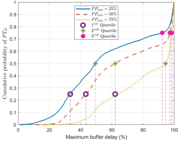
Fig. 5. Cumulative probability of maximum buffer delay  $PT_D$  for the optimal transmission window  $TW_O$  where the minimum power saving requirement  $PP_{min}$  is set to 25%, 50%, and 75%.
