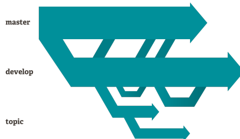
Figure 4.1: Typical Git workflow
