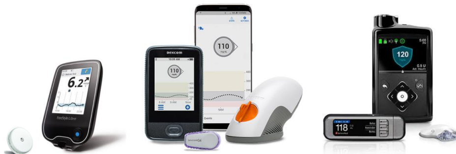
Figure 5. Photos of glucose sensors. Left photo shows the FreeStyle Libre sensor and reader from Abbott. Middle photo shows Dexcom G6 with applicator, receiver and a smart phone from Dexcom. Right photo shows the MiniMed 670G system with sensor, BG meter, and insulin pump from Medtronic. (Images downloaded from www.freestylelibre.no , www.dexcom.com , and www.medtronicdiabetes.com , October 2019).
