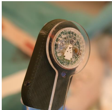
Figure 15. Photo of the custom-made holder with the FreeStyle Libre sensor and LimiTter attached. The LimiTter is the dark green rounded shape and was fixed to the outside of the abdominal wall to collect sensor signals from the IP inserted FreeStyle Libre sensors. Photo by Patrick C. Bösch.
