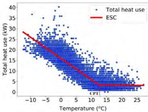
Figure 1: An example of the energy signature curve for the considered apartment building (Csoknyai et al., 2019).
