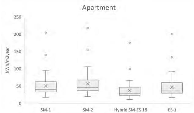
Figure 10 Boxplots of annual specific energy use for DHW decomposed with different methods in 58 apartment blocks.
