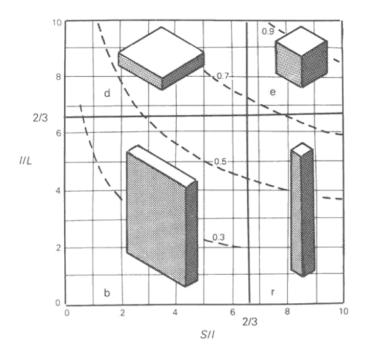
Figure 2.5: Classification of particle shape depending on the length of long (L, length), intermediate (I, width) and short (S, thickness) axes (Lindholm 2012, after Zingg 1935).
