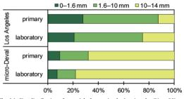
Fig. 14. Size distribution of material after testing by Los Angeles (N = 29) and micro-Deval (N = 25) methods for primary crushed material and laboratory crushed material.
