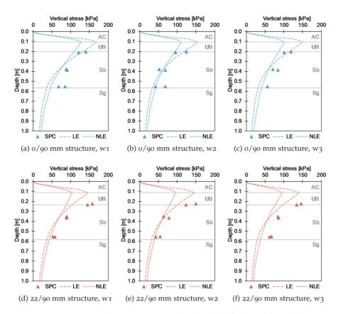
Figure 4.12: Comparison between measured and modelled induced vertical stress as a function of depth at the end of each groundwater phase. w1 – 500 000 load repetitions; w2 – 930 000; w3 – 1 233 000. Horizontal lines indicate layer boundaries.
