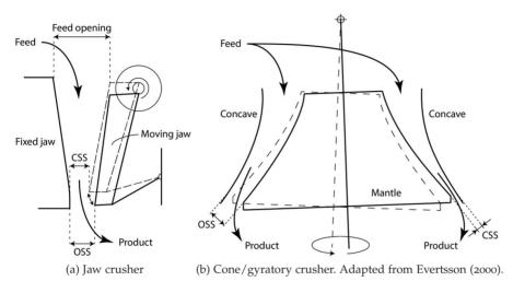
Figure 2.2: The principles of common compressive crushers.
