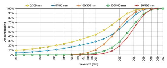
Fig. 1. Feed material particle size distributions from image analysis. Each line represents average values from all tested materials of each size fraction.
