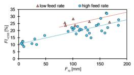
(a)  $FI_{<CSS}$  vs  $F_{10}$ , differentiated by feed rate. Regression analysis combining  $FI_{<CSS}$ ,  $F_{10}$  and feed rate:  $r^2 = 0.713$
