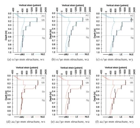
Figure 4.11: Comparison between measured and modelled induced vertical elastic strain as a function of depth at the end of each groundwater phase. w1 – 500 000 load repetitions; w2 – 930 000; w3 – 1 233 000. Horizontal lines indicate layer boundaries.
