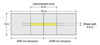
Figure 3.5: Outline of HVS test pit seen from above.
