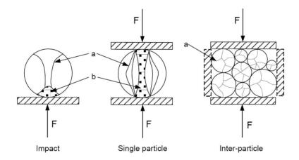
Figure 2.1: Crushing principles – impact crushing, single-particle compressive crushing, and inter-particle compressive crushing (Bengtsson, 2009). a = principal cracks; b = fines generated on account of breakage.
