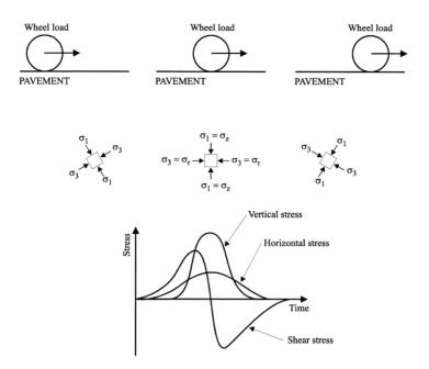
Figure 2.8: Development of stress in unbound layers beneath a moving wheel load (Lekarp and Dawson, 1998).
