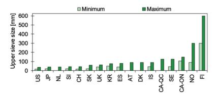
Figure 4.2: Upper sieve size limits for subbase materials.
