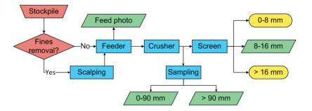
Figure 3.1: Process flowchart for the full-scale crushing test, including sampling.
