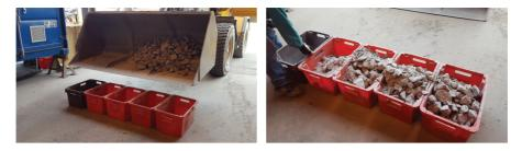
Figure 3.3: Method for collection of product samples from wheel loader bucket.
