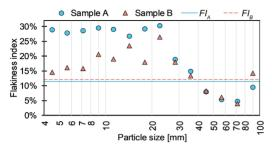
Fig. 20. Comparison of individual fraction FI (points) for two test materials of similar  $FI_{4-100}$  (lines).
