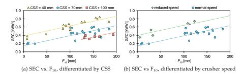
Figure 4.3: Specific energy consumption vs. lower size of feed material ( $F_{10}$ ), differentiated by CSS and crusher speed. Regression analysis combining SEC,  $F_{10}$ , CSS and speed:  $r^2 = 0.83$ .
