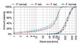
Fig. 6. Feed (F) and product (P) particle size distribution curves for 100/400 mm samples tested at normal and reduced speed. Each line represents the average of minimum 3 parallel tests.
