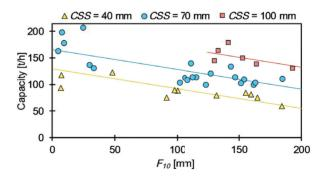
Figure 3.4: Multiple linear regression example from Paper C: Crusher capacity depending on lower feed size  $F_{10}$  and closed side setting CSS,  $r^2 = 0.77$ .
