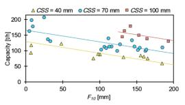
Fig. 3. Capacity vs  $F_{10},$  differentiated by CSS. Combined regression analysis:  $r^2\,=\,0.77.$
