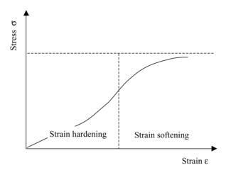
Figure 2.10: Stress-strain behaviour of unbound granular materials (Werkmeister, 2003).
