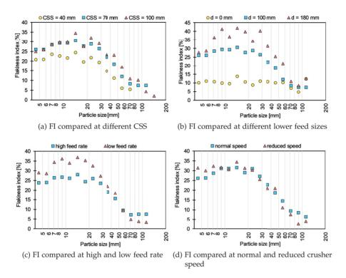
Figure 4.6: Particle shape measured as FI for individual particle size fractions.
