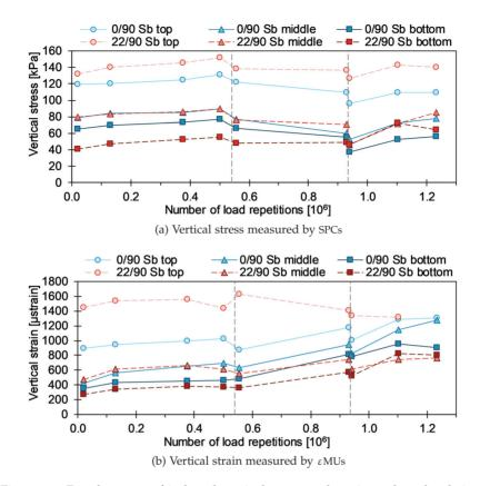
Figure 4.9: Development of induced vertical stress and strain at three levels in the two subbase layers during APT. Vertical dashed lines indicate GWT raises.
