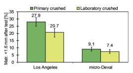
Fig. 13. Mechanical properties measured before and after laboratory crushing (average values). The error bars indicate maximum and minimum values for each data set (N = 38 for each column).
