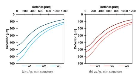
Figure 4.8: Back-calculated deflection from FWD, adjusted to 10 °C.
