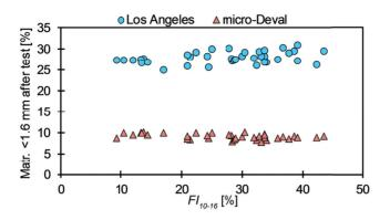
Figure 4.5: Mechanical properties vs. flakiness index for particles in the size range used in mechanical testing.
