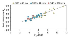
**Fig. 9.** Reduction ratio  $R_{80}$  as a function of the ratio between the upper size for the feed material  $F_{90}$  and the crusher setting *CSS*;  $r^2 = 0.842$ .
