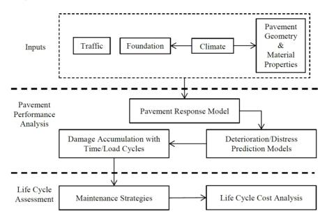
Figure 2.7: Flowchart for a mechanistic-empirical pavement design procedure (Ahmed, 2014).
