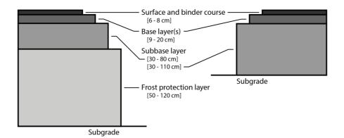
Figure 2.6: Outline of typical Norwegian pavement structures with and without frost protection layer.
