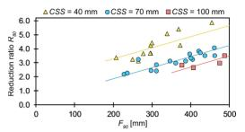
**Fig. 8.** Reduction ratio  $R_{80}$  vs. the upper size for the feed material  $F_{90}$ , differentiated by closed side setting *CSS*. Regression analysis combining  $R_{80}$ ,  $F_{90}$  and *CSS*:  $r^2 = 0.808$ .
