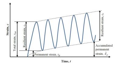
Figure 2.9: Development of resilient and permanent strain during traffic loading (Rahman, 2015).
