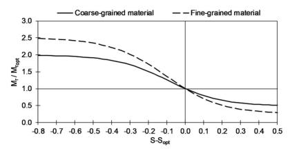
Figure 2.11: Ratio of resilient modulus as a function of change in degree of saturation. Adapted from ARA Inc. (2004).
