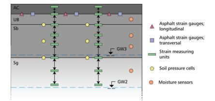
Figure 3.7: Instrumentation of pavement structures in APT. Size of symbols and horizontal distance between sensors not to scale.
