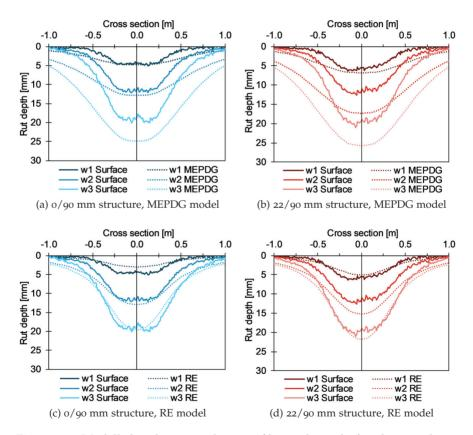
Figure 4.15: Modelled and measured rut profiles at the end of each groundwater phase (550 000, 935 000 and 1 233 000 load repetitions).
