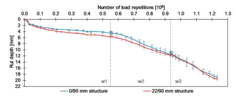
Figure 4.10: Rut development during APT. Each line represents the average of three laser profiles; error bars show max/min measurements. Dashed vertical lines indicate GWT phase transitions.
