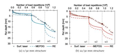
Figure 4.14: Modelled rut development compared to surface laser measurements. Dashed vertical lines indicate GWT phase transitions.
