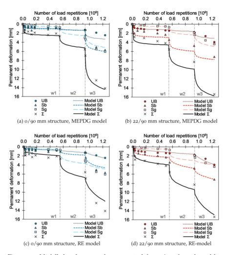
Figure 4.13: Modelled and measured permanent deformations for unbound base (UB), subbase (Sb) and upper 15 cm of subgrade (Sg). Dashed vertical lines indicate GWT phase transitions.
