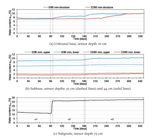
Figure 4.7: Registered volumetric water content from sensors in unbound base, subbase and subgrade during APT. Start and end of groundwater adjustment periods indicated by vertical dashed lines.
