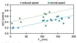
**(b)** *SEC* vs  $F_{10}$ , differentiated by crusher speed
