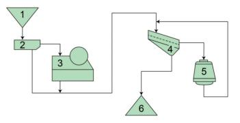
Figure 2.3: Example aggregate production process flowchart for 0/90 mm subbase. 1 – Feed stockpile; 2 – Feeder; 3 – Primary jaw crusher; 4 – Screen; 5 – Secondary gyratory crusher; 6 – Product stockpile. Adapted from Eloranta (2009).
