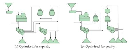
Figure 2.4: Examples of process optimisation for either capacity or quality. Adapted from Eloranta (2009).
