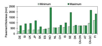
Figure 4.1: Minimum and maximum pavement thicknesses for annual average daily traffic (AADT)  $\approx$  10 000.
