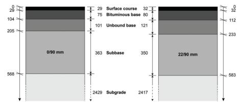
Figure 3.6: Outline of pavement structures in APT. Depth and layer thicknesses measured in mm. AC – asphalt concrete; UB – unbound base; Sb – subbase; Sg – subgrade.
