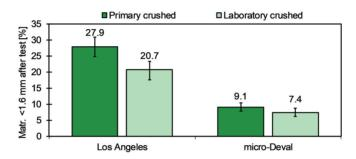
Figure 4.4: The impact of sample preparation by laboratory crushing on measured mechanical properties (average values). The error bars indicate maximum and minimum values for each data set (N = 38 for each column).
