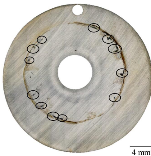
Figure 5-1. LOM capture of UNS S39274 specimen after crevice corrosion test with the PD-GS-PD technique in 3.5 wt.% NaCl at 60°C. Circles indicate crevice corrosion attacks identified with the IFM.
