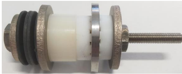
Figure 4-2. Multi-crevice assembly used in this thesis, as described in ISO18070 [128].
