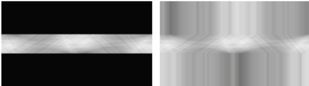
Figure 5. Sinogram images of a scan with higher FOV than the object size. Left one is the original processing, while at right one an easy trick has been applied for future convenience. [19]
