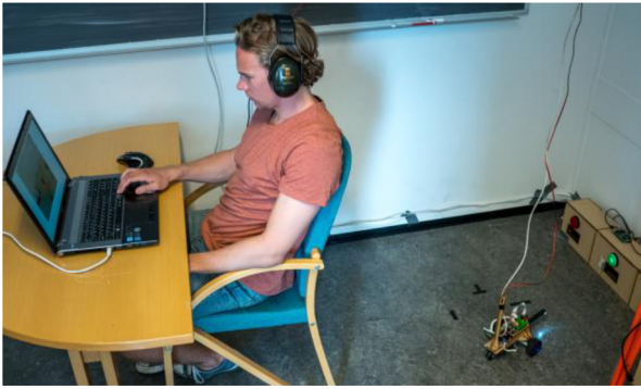
Fig. 3. Experiment setup. The participant can only see the robot through the display provided on the laptop screen, which is a first-person camera view.
