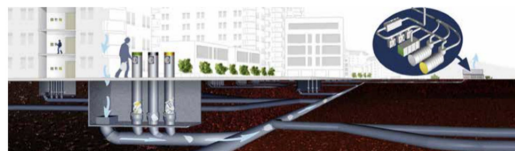
Figure 5. Smart waste collecting system.
