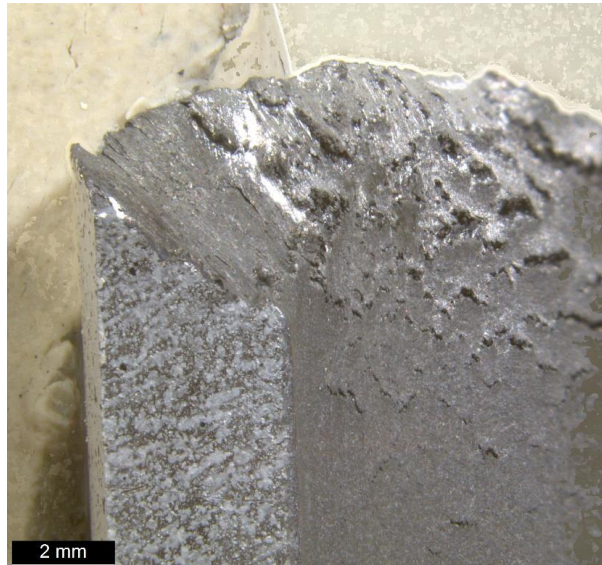
Figure 4.1.11. Side view of a failed specimen. The shear crack propagation, the multitude of diffused secondary cracks and the final plastic tearing executed at the end of the test are distinguishable.
