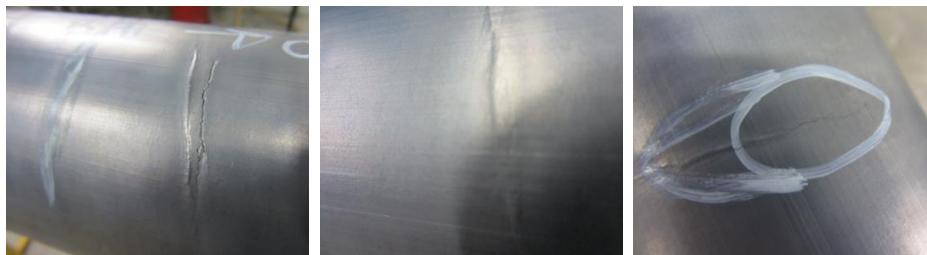
Fig. 3.3.9. (Left) Outside of a (failed) XLPE power phase after 15,000 cycles at 1.1 % \Delta\varepsilon ; (Center) Outside of a (run- out) XLPE power phase after 25,000 cycles at 0.4 % \Delta\varepsilon ; (Right) Outside of a (failed) XLPE power phase after 30,000 cycles at 0.4 % \Delta\varepsilon .
