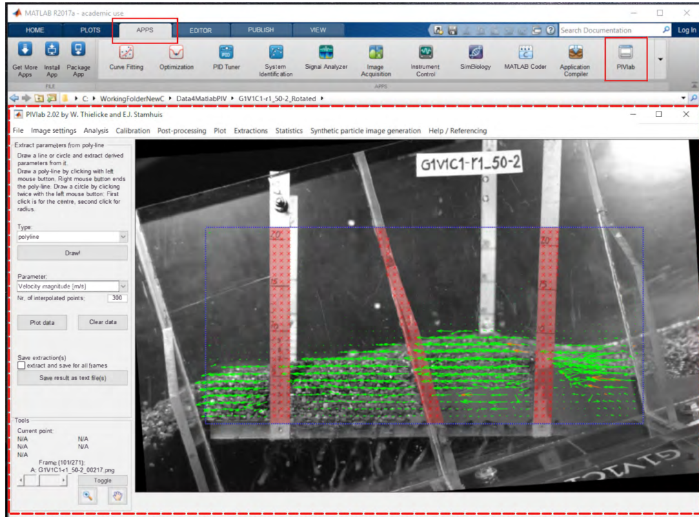
Fig. 3.14: The PIVLab App of MATLAB being used for determination of flow velocity over the screen (Flow direction is from right to left)
