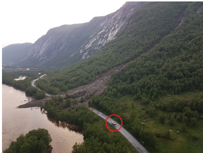
Fig. 1.1: Example of coastal debris-flow: Mjøland, Norway (02.06.2016). A Firetruck is circled for scale. [Photo: NPRA and Multiconsult]
