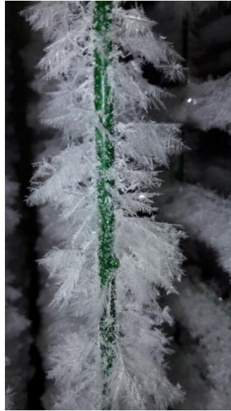
Figure 3.1: Synthetic snow crystals growing on steel wire. Courtesy of M. Dahl Fenre at the Norwegian University of Science and Technology (NTNU), Trondheim.
