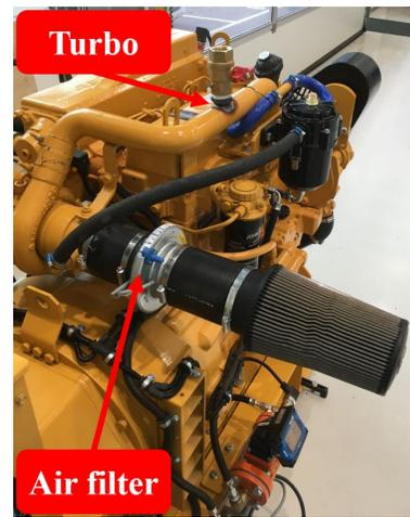
Fig. 4. The restriction and bleed device used to provoke the air filter and turbo fault, respectively.
