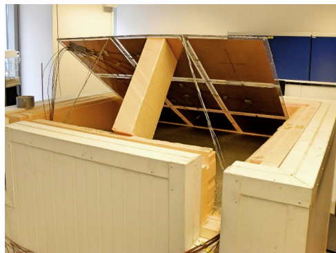
Figure 12. Heat flux plates at the top of the sample (Rieksts et al., 2017 [27]).
