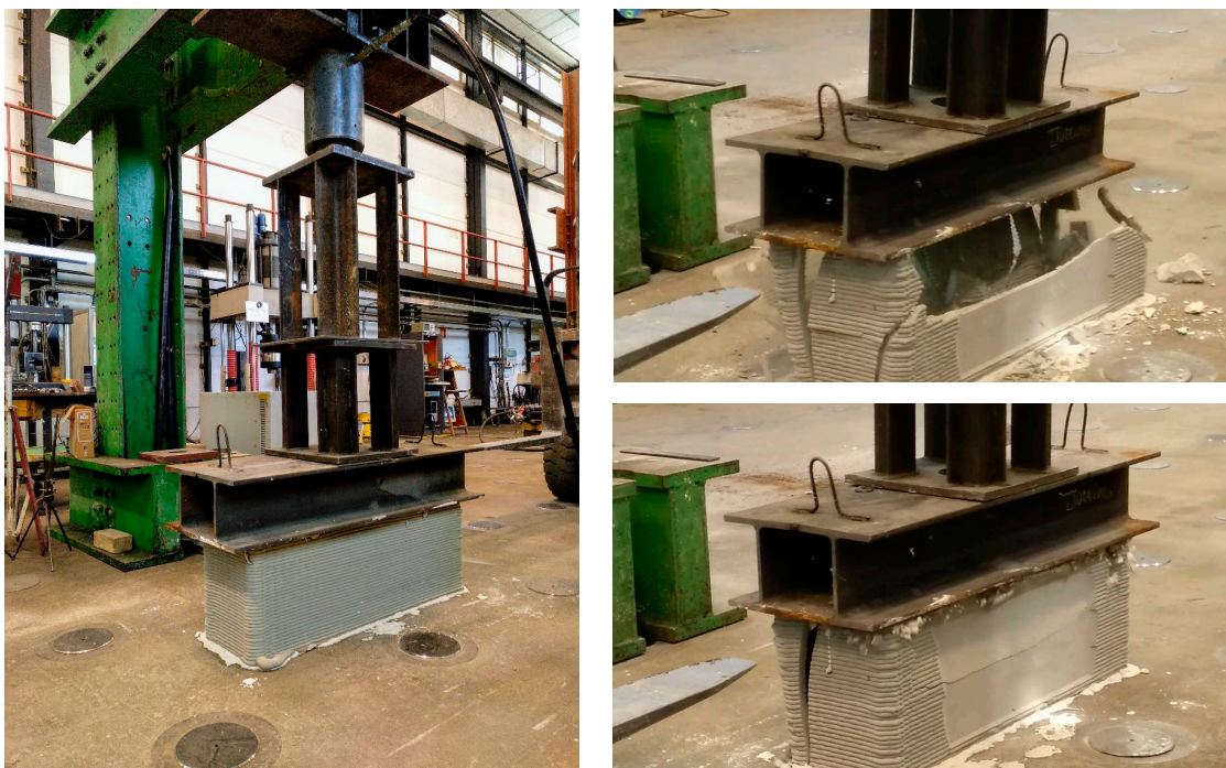
Figure 21. Mechanical testing of a HINDCON project 3D-printed element.
