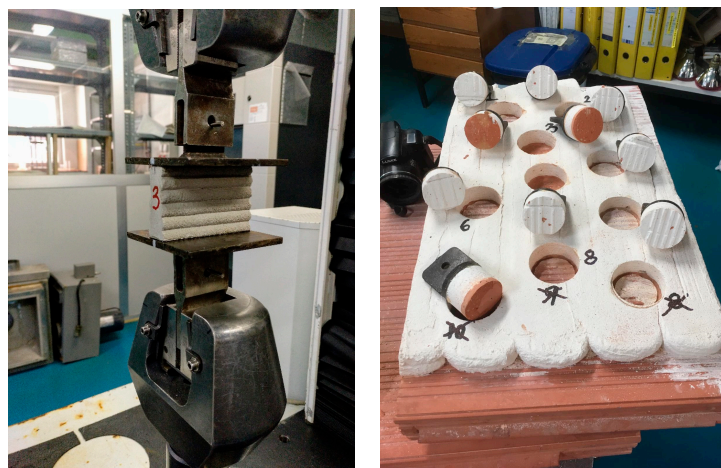
Figure 12. Pull-off adhesion test between layers (left) and to the substrate (right); HINDCON and 3DCONS projects.
