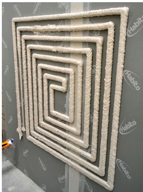
Figure 3. Vertical printing test with material developed within the 3DCONS project.
