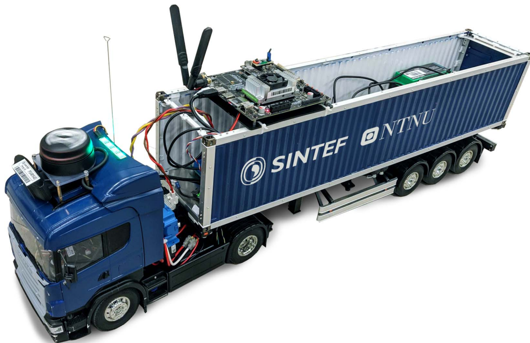
Figure 1 Small-scale truck model equipped for autonomous driving and wireless charging
