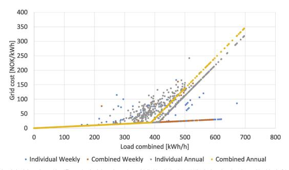
**Fig. 5.** Resulting hourly load dependent grid tariff costs, i.e., load dependent price multiplied by the load, in NOK/kWh plotted against the combined load of Campus 1 (C1) and Campus 2 (C2) for the individual weekly (IW) scheme (blue), combined weekly (CW) scheme (orange), individual annual (IA) scheme (gray), and combined annual (CA) scheme (yellow). (For interpretation of the references to colour in this figure legend, the reader is referred to the Web version of this article.)
