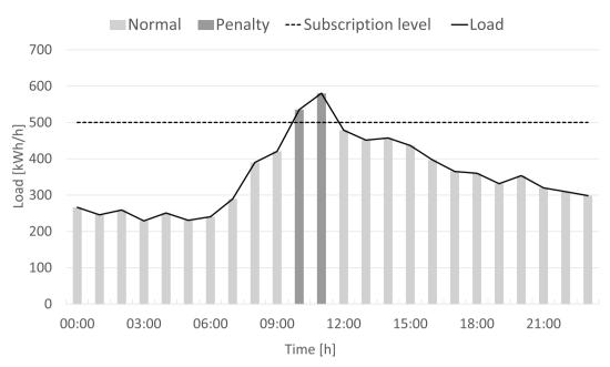
Fig. 1. Illustration of the 'subscribed capacity' grid tariff scheme. The illustration shows an example of measured hourly load over 24 h for the combined load of Campus 1 (C1) and Campus 2 (C2) and a combined subscription. The horizontal line represents the subscription level which causes a penalty charge for hours 11 and 12 (load exceeds subscribed level).
