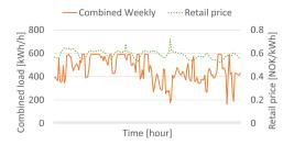
(b) Resulting cost-optimal load (orange) with the combined weekly (CW) scheme.
