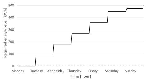
**Fig. 2.** The lower bound for energy that must be charged by time  $t \in \mathcal{T}$  to battery electric vehicles. This offers flexible charging in every time-step with some constraints (daily demands).
