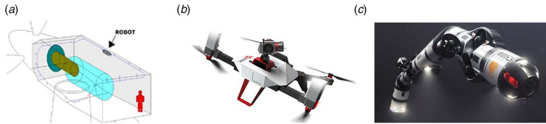
Fig. 7 Tools for enabling inspections in areas with difficult access [54–56]: (a) a robot for drivetrain inspection, (b) a remotely piloted aircraft system for blade inspection, and (c) underwater snake robot vehicle
