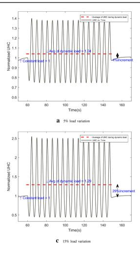
Fig. 6 Unburned hydrocarbon variation (modeling Type E)
