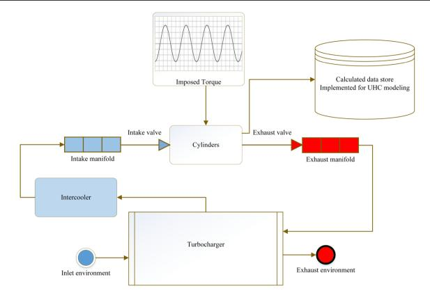
Fig. 3 Engine modeling flowchart
