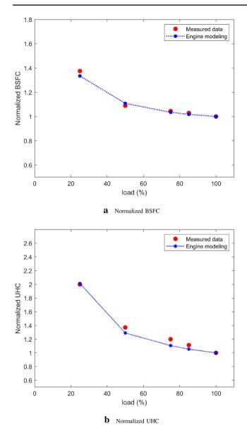
Fig. 4 Simulated and measured BSFC and UHC versus load at rated speed
