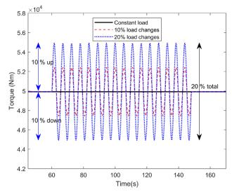
Fig. 5 Imposed dynamic load
