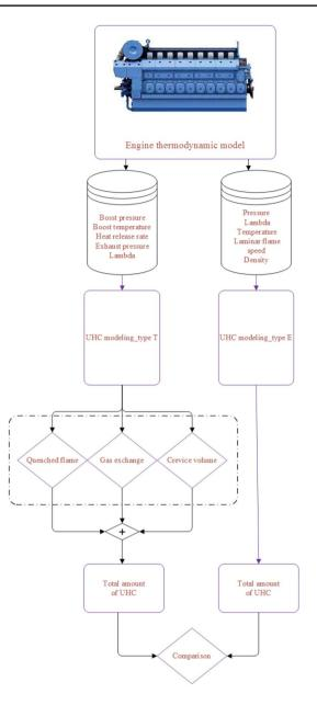
Fig. 1 Emission modeling flowchart
