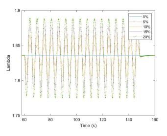
Fig. 12 Air-fuel ratio variation during dynamic load
