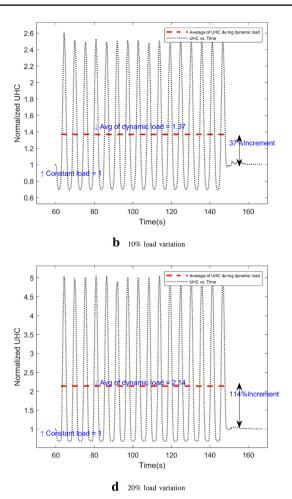
Fig. 8 Unburned hydrocarbon variation (modeling Type T)
