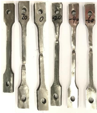
(b) Fractured specimens (The first specimen to the left was not stretched, and the remaining specimens were stretched under low temperature.)
