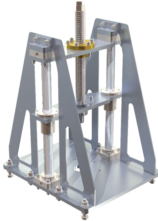
Figure 27 In-house designed assembly jig
