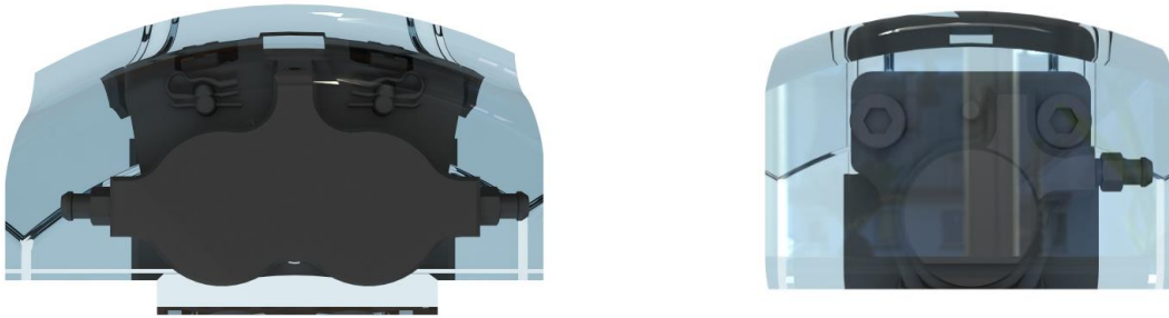
Figure 13 Front and rear caliper design spaces seen in transparent material ISR calipers seen in grey.
