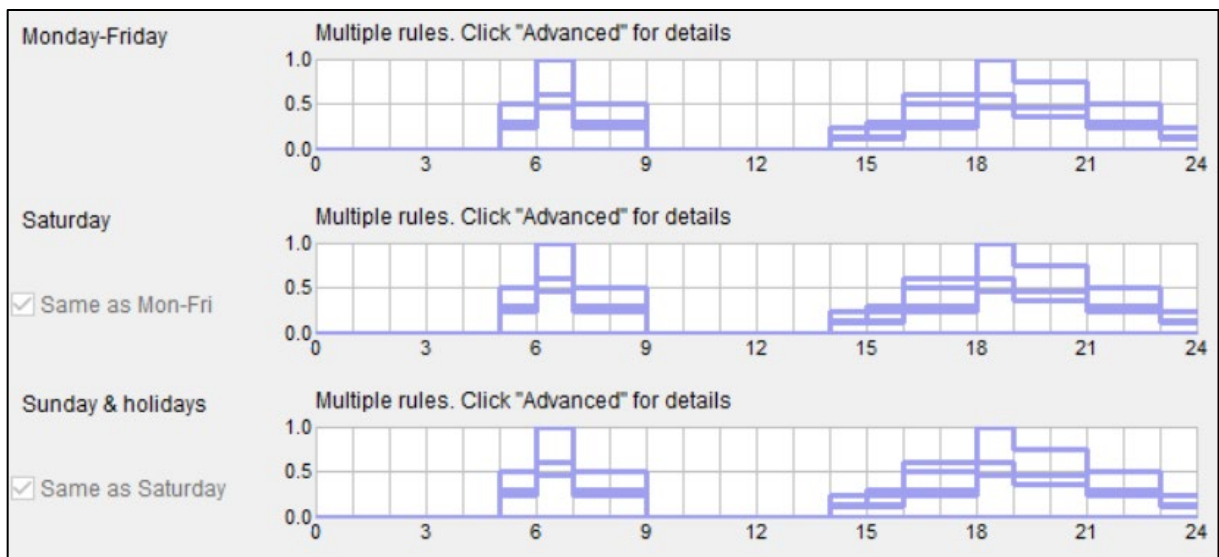
Figure 29 Lighting distribution schedule based on NS:3031(2016) and finish survey (Karlsen et al., 2020).
